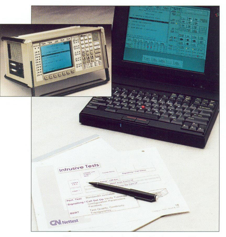
The remote control option allows the placement of the DST 2000(s) in unmanned or partially manned offices and controlled from a central diagnostic centre via an IBM or compatible personal computer. The PC can "talk" to the DST 2000 via leased, dial or X.25 connections.
