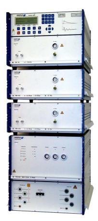
The PSURGE 8000 Test System can perform all the programming functions required to perform **ANSI C62.41** and **UL 1449** testing without the need of a control computer.
