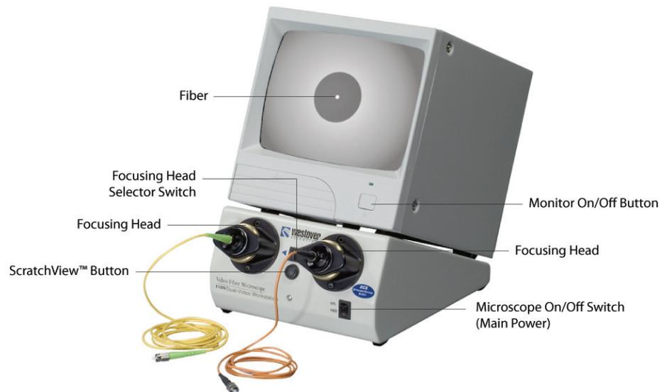
The FVDW Series microscopes utilize coaxial illumination to provide the user with a critical view of fine scratches, making them the ideal choice for factory post-polish inspection, component assembly, and QC environments. The FVDW systems feature an attached 9" monitor that is inclined backward 22.5° and accept all FMA-Series adapters. Each microscope has two heads, ideal for inspecting:
