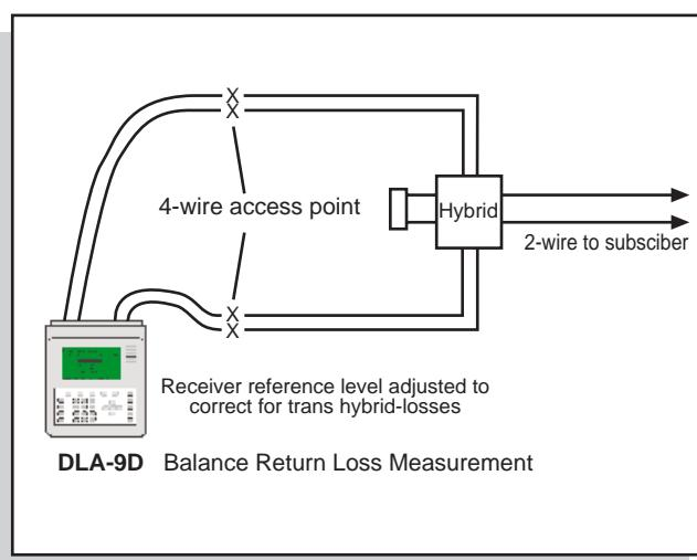
Having determined the trans-hybrid loss the receiver should be set in relative mode and the correction applied to the Rx Reference Level to enable the Balance return loss measurement to be made directly.
