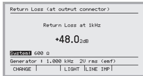
It is desirable for 2-wire return loss to be a high figure indicating a good impedance match between the CPE and the network.
