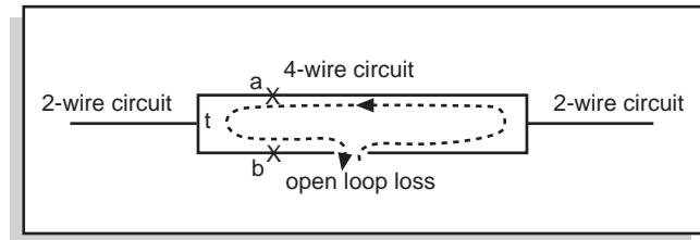
**“Semi-Loop Loss:** The transmission loss between points ‘a’ and ‘b’ of the 4-wire termination independent of whether there exists or not a physical point ‘t’.”
