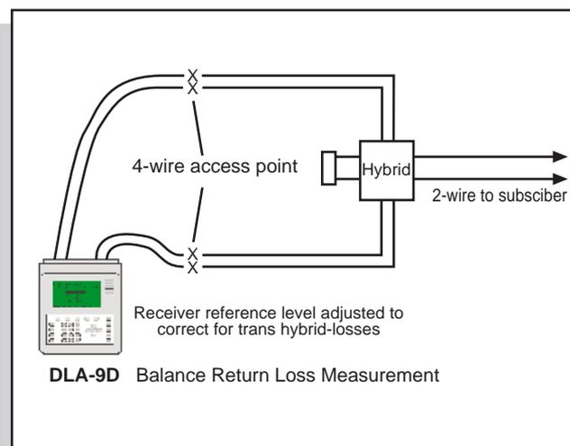
Having determined the trans-hybrid loss the receiver should be set in relative mode and the correction applied to the Rx Reference Level to enable the Balance return loss measurement to be made directly.
