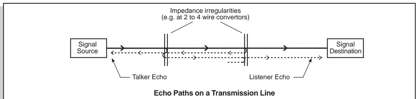
Impedance mismatches in communications circuits cause problems because signals are reflected back to the source from each mismatch. This can result in a loss of power transfer and interference with, or corruption of, the signal.
