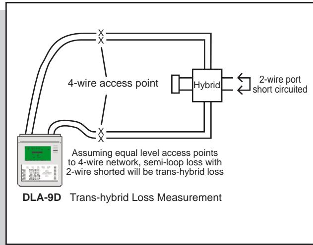
The trans-hybrid loss is determined by shorting the 2-wire port of the hybrid and measuring the circuit loss on the 4-wire side. In the ideal case this would be -6dBm.
