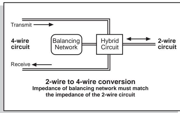
For the hybrid to work correctly the impedance of the balancing network should match that of the 2-wire circuit. In practice the 2-wire impedance depends on the loop length and conditions so it is difficult to balance correctly. This results in echoes and return losses on both sides.
