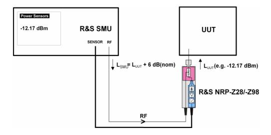
Typical measurement setup with an R&S NRP-Z28/-Z98 level control sensor and an R&S SMU signal generator. The power level incident on the UUT can directly be read off from the "Power Sensors" menu.
