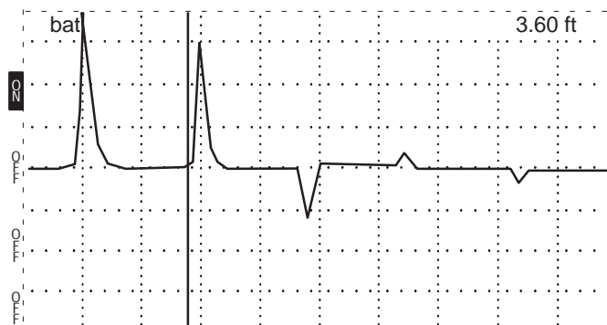
Figure B-4: Cursor at End of 10-foot Cable, V_p Set to .30
