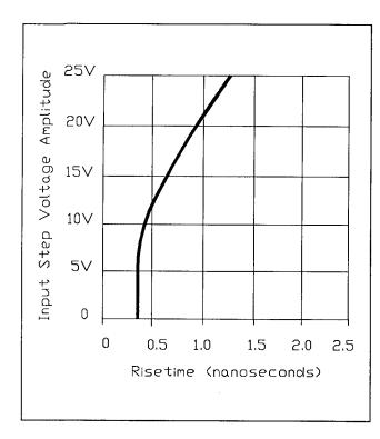
Figure 2-1. Typical linear operating region for step inputs.
