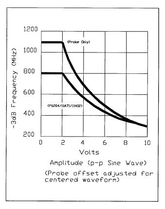
Figure 2-2. Typical -3dB frequency versus amplitude.
