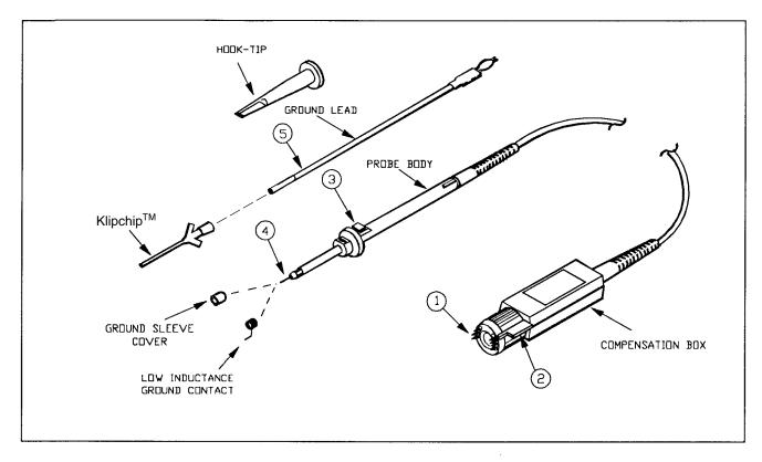
Figure 2-5. Controls, connectors and probe accessories.
