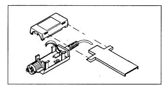
Figure 6-1. Compensation box disassembly.
