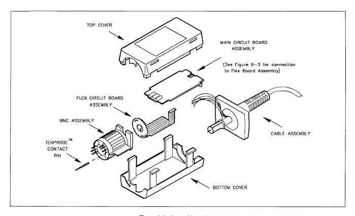
Figure 6-2. Assembly replacement.
