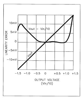
Figure 1-3. Typical Linearity Curve.
