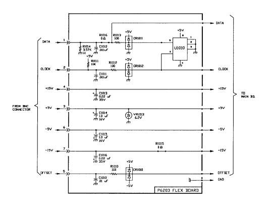
Figure 7-2. The P6204 Flex board schematic.
