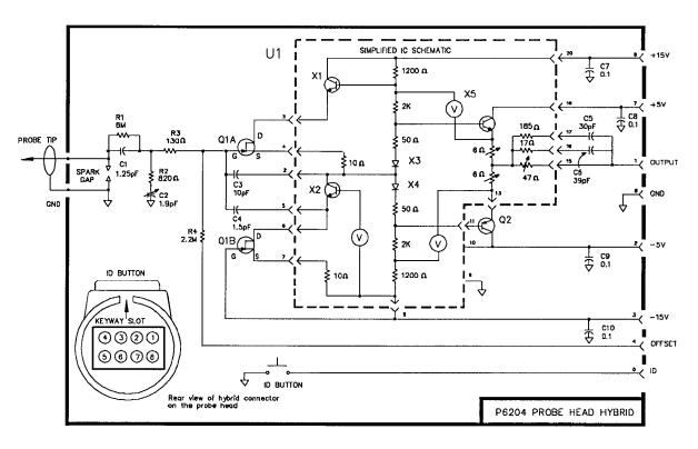
Figure 7-3. The P6204 Probe Head board schematic.
