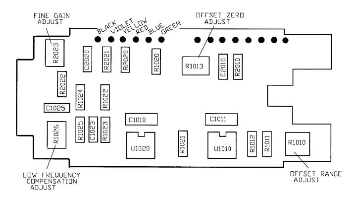
Figure 7-4. The Main Circuit board component layout.
