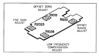
Figure 4-1. Compensation box adjustment locations.
