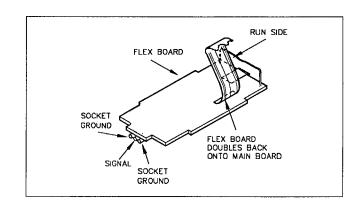
Figure 6-3. Flex Circuit board replacement.
