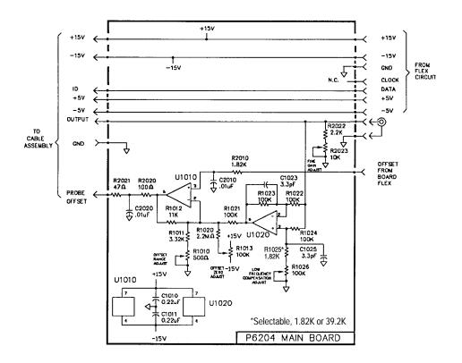
Figure 7-1. The P6204 Main board schematic
