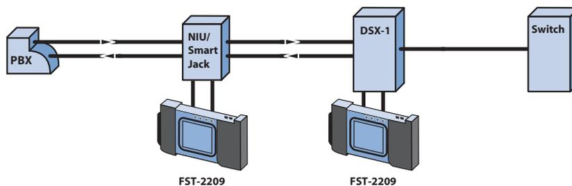
The FST-2209 quickly and effectively measures the quality of voice transmission on the network circuit
