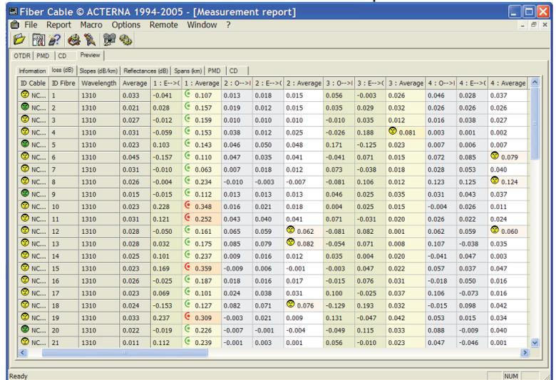
Step 4: Incorrect, missing and out-of-range results pointed out
