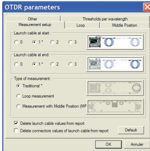
Figure 3: OFS-200 FiberCable: OTDR report parameter setup
