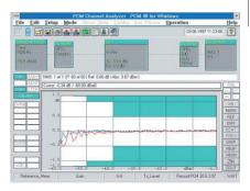
The fall-off in gain can be clearly seen. The blue trace was recorded on commissioning the system, the red trace at a later date. The "DIFF RESLT" function determines the difference between the two traces. The zoom function and cursors allow every detail to be examined.
