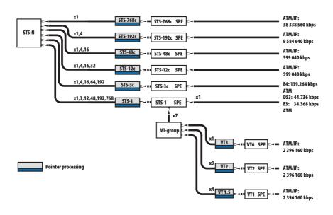
figure 10 SONET multiplexing scheme
