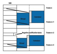
This allows for the free insertion in time of user signals into the next higher frame structure in the form of virtual containers without the need for larger buffers. However, changes in the phase location of the virtual container relative to the superior frame can be corrected by appropriate pointer actions. Such changes and shifts in phase can be caused by changes in propagation, delay in the transmission medium or by non-synchronous branches in the real network.
