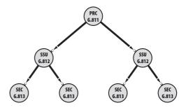
The clock signal is regenerated in the SSUs and SECs with the aid of phase-locked loops. If the clock supply fails, the affected NE switches over to a clock source with the same or lower quality. If this is not possible, the NE switches to holdover mode. In this situation, the clock signal is kept relatively accurate by controlling the oscillator, applying the stored frequency correction values for the previous hours and taking the temperature of the oscillator into account.
