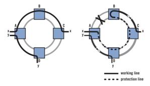
figure 18 Two-fiber bidirectional line-switched ring (BLSR) working line protection line
