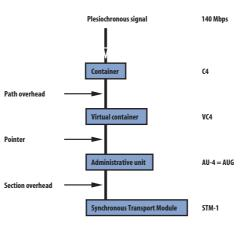
ATM signals can be transported in the SDH network in C11,C12,C3, and C4 containers. Since the container transport capacity does not meet the continually increasing ATM bandwidth requirement, methods have been developed for transmitting the ATM payload in a multiple (n) C-4 (virtual or contiguous concatenation). As an example, a quadruple C-4 can be transmitted in an STM-4 (see section on "Contiguous concatenation").
