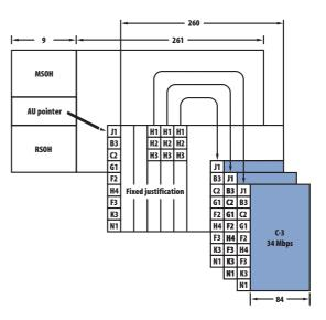
SDH multiplexers are controlled from a highly accurate central clock source running at 2.048 MHz. Pointer adjustment may be necessary if phase variations occur in the real network or if the connection is fed through the networks of different providers. The AU pointer can be altered in every fourth frame with prior indication. The virtual container is then shifted by precisely three bytes. Pointer activity is therefore a good indication of clock variations within a network.
