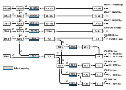
figure 9 Mapping in SDH
