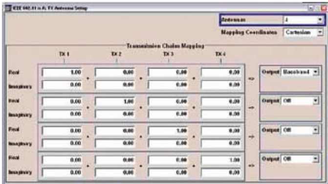
Up to four TX signals can be generated and added up with complex weighting factors. This enables convenient testing of WLAN IEEE 802.11n receivers with up to four antennas under static fading conditions.
