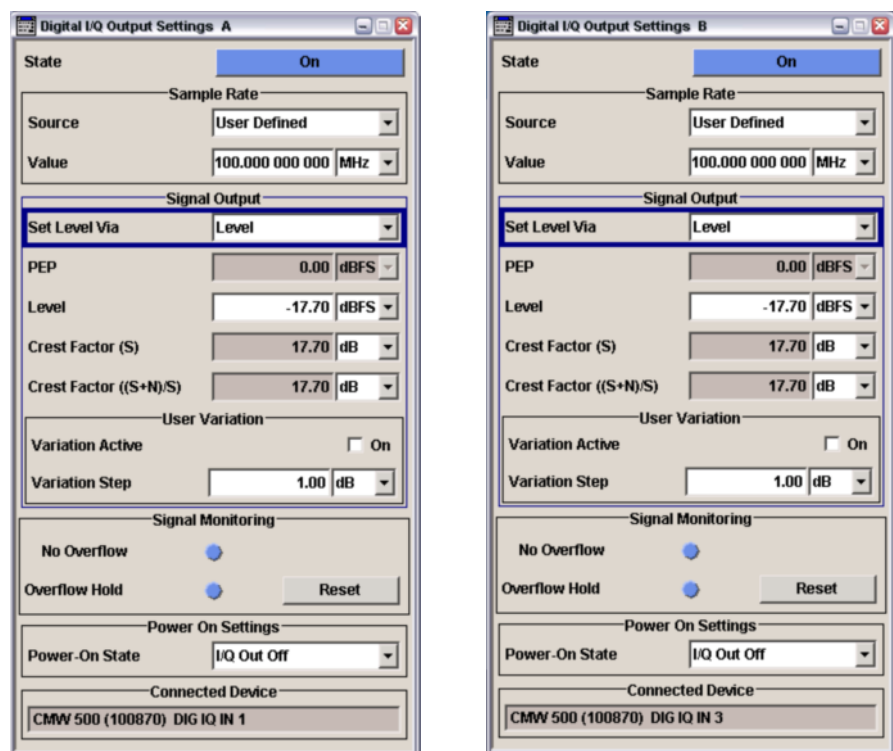
Figure 18: AMU digital baseband output settings
