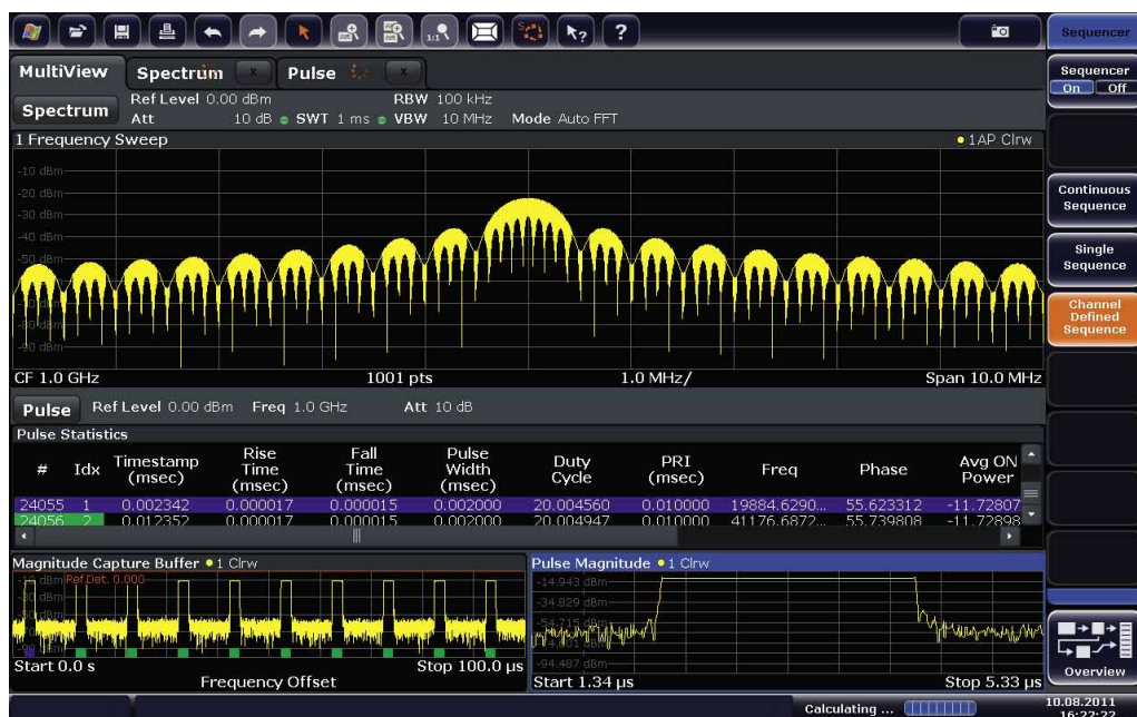
FIG 3 The R&S®FSW's MultiView function simultaneously displays the results of multiple measurement applications in separate windows.
