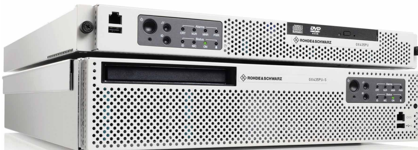
FIG 1 The modular R&S®GX435 multichannel signal analysis solution is built from appropriate quantities of the two basic components. The R&S®GX435PU-S component for processing and storage (bottom) controls the R&S®GX435, computes the DDCs as well as the signal detectors in the configuration without hardware acceleration, and serves as a recording/replay unit. The R&S®GX435PU component for processing (top) processes up to eight signals simultaneously by performing classification, demodulation and decoding.
