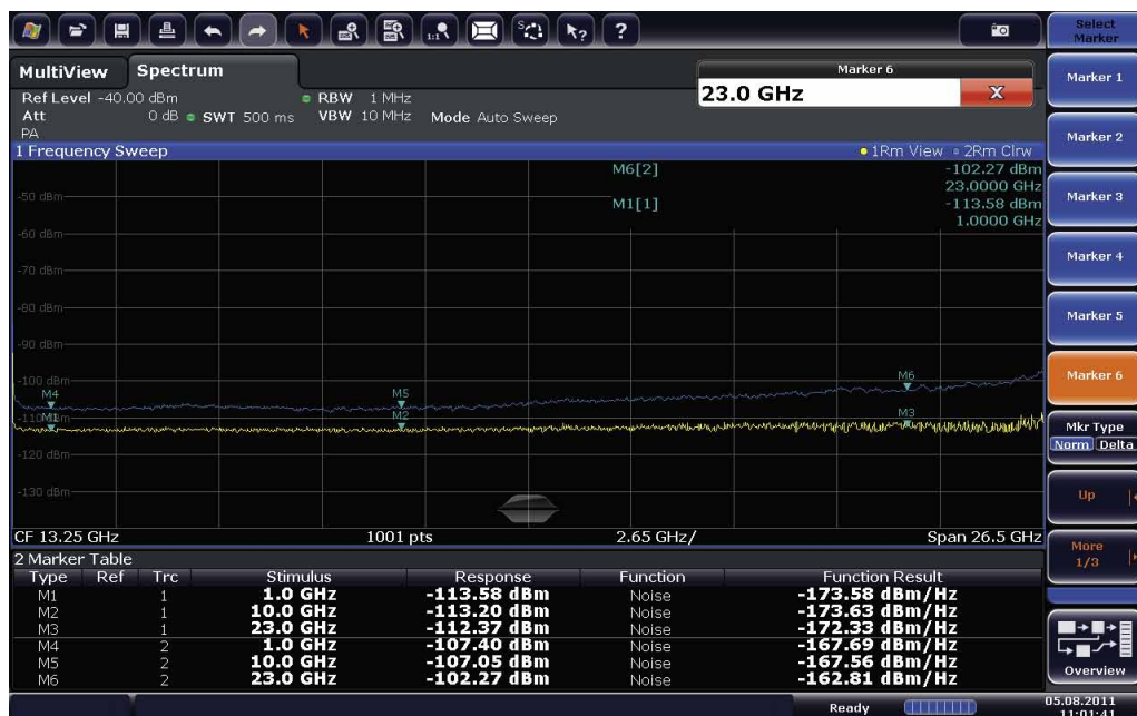
FIG 7 Displayed average noise level (DANL) with preamplifier and noise cancellation switched on.
