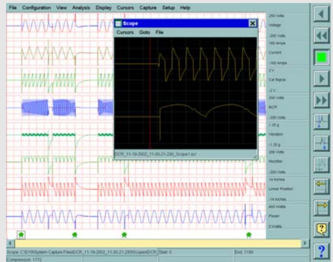
▲ Embedded Scope Capture: Data acquisition can be performed in the background without interrupting real-time recording. Internal scope captures and optional scope card captures can be embedded in standard data captures, giving you trend recording and triggered captures in one file!*
