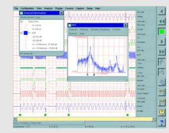
**On Screen Analysis:** On screen cursors let you make precise, error-free waveform measurements. The FFT analysis window gives you access to your data in the frequency domain – ideal for power or audio applications. Embedded scope captures can be reviewed, along with waveform data, at the touch of a button.
