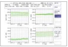
Measurement example of EDFA gain and wavelength dependency of NF (Measurement results displayed on the AQ8423Z's screen)
