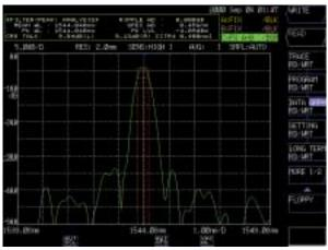
Measurement example of transmission characteristics of WDM filter
