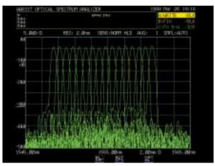
Measurement example of transmission characteristics of 16-channel AWG
