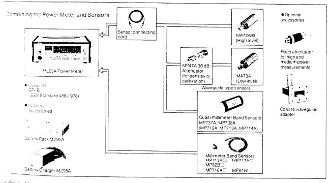
Power Meter ML83A is a digital power meter of high permission with a microprocessor, having multiple functions for the variety of applications. In particular, it has the averaging on and is capable of reading low levels with high accurate GP-IB interface is available by option for automatic
