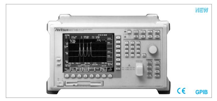
The MS9710B is a diffraction-grating spectrum analyzer for analyzing optical spectra in the 0.6 to 1.75  $\mu m$  wavelength band. In addition to uses such as measurement of LD and LED spectra, it has functions for measuring the transmission characteristics of passive elements such as optical isolators, as well as the NF/Gain of optical fiber systems.
