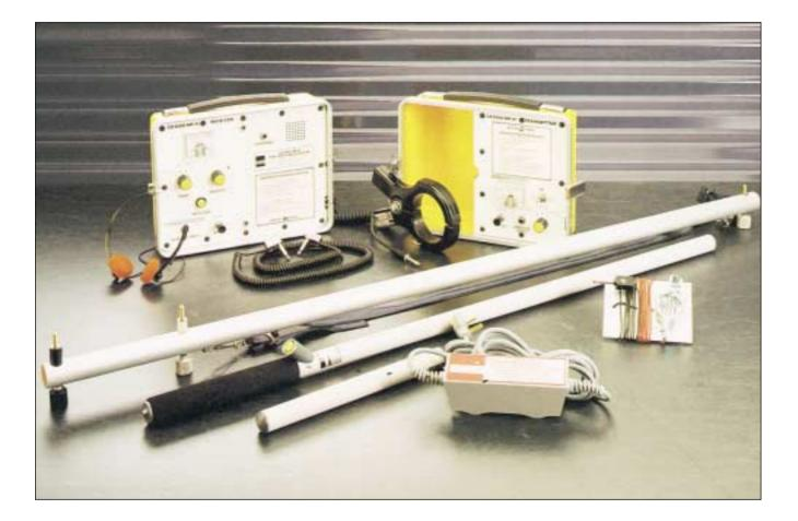
The CZ6000 MKIII Pipe & Cable Locator is a compact, portable instrument for the detection and location of buried pipes and cables. It consists of a directional radio transmitter and receiver that can be used either coupled together mechanically as a metal detector, or separately for precise location of a targeted line. It comes complete with conductive connecting wires and clips, and headphones, and is powered by readily available 1.5V AA batteries.
