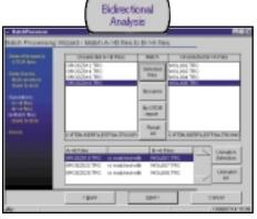
When performing OTDR bidirectional averaging, all acquisitions from both directions of a cable can be matched in one operation, either manually or automatically.
