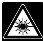
Figure 2-7. Laser Radiation Hazard Sticker on Side Panel
