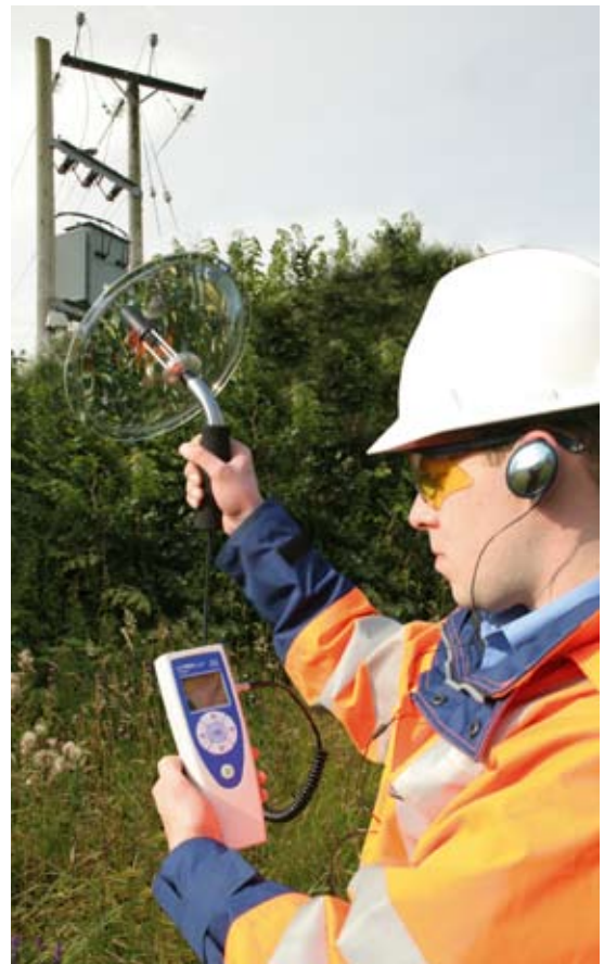
Listen for PD activity in overhead assets with the UltraDish™ add-on.
