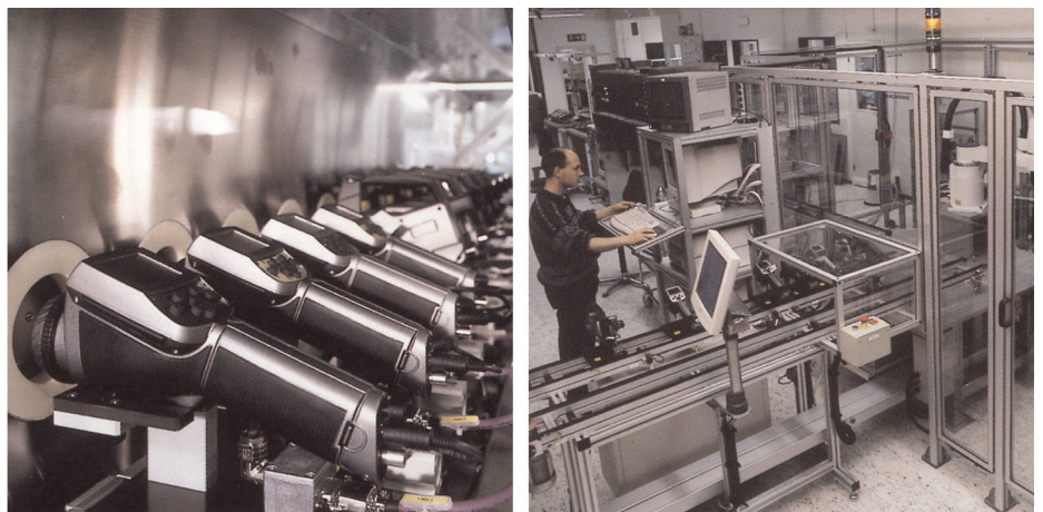
Figure 25.5 LEFT: Testing of infrared cameras in the climatic chamber; RIGHT: Robot used for camera testing and calibration
