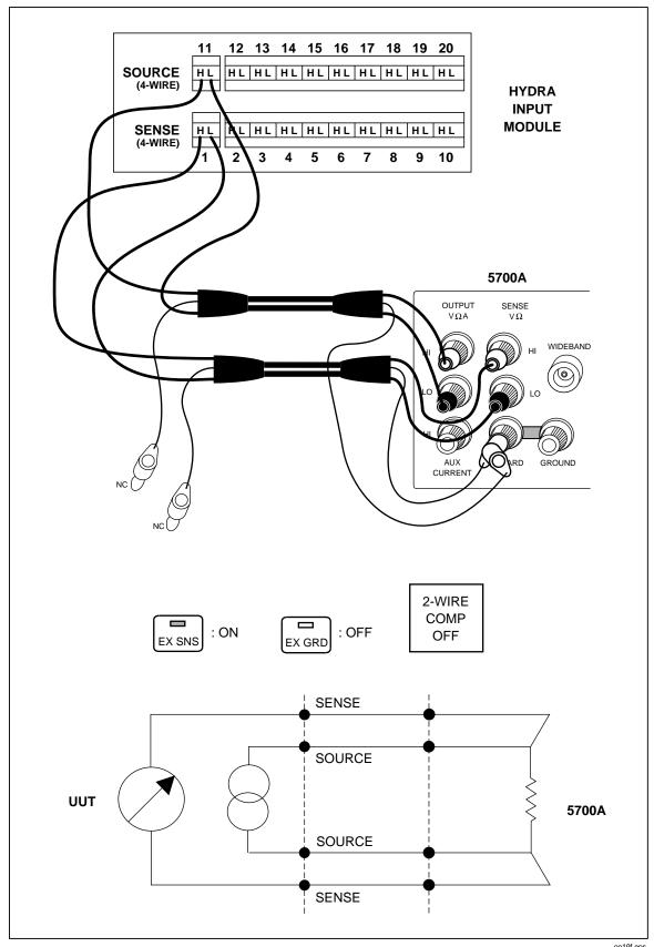
Figure 6-2. 4-Terminal Connections to 5700A
