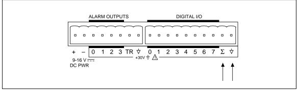
Figure 3-4. Totalizing Connection
