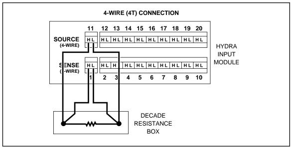
Figure 6-3. 4-Terminal Connections to Decade Resistance Box
