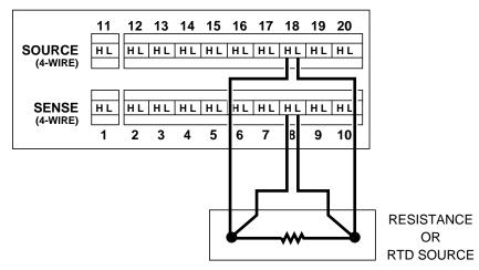
USE H AND L TERMINALS FOR TWO CHANNELS ON REAR PANEL INPUT MODULE. CONNECTIONS FOR CHANNEL 8 SHOWN HERE WITH CHANNEL 18 PROVIDING ADDITIONAL TWO CONNECTIONS.
