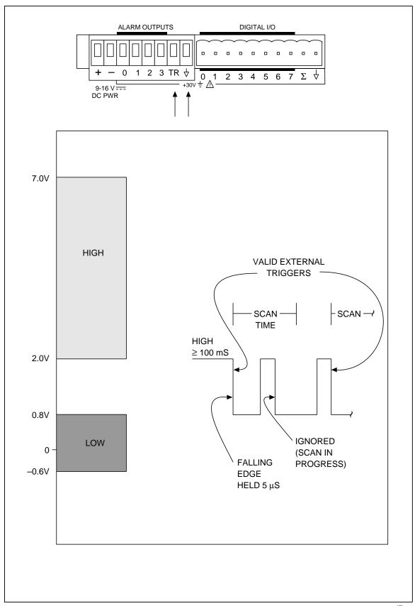
Figure 5-1. External Trigger Timing
