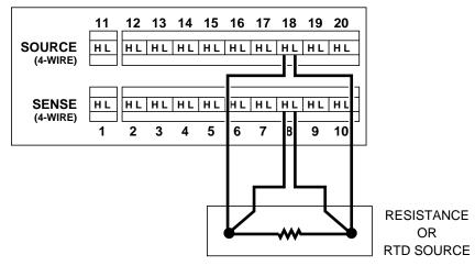
USE H AND L TERMINALS FOR TWO CHANNELS ON REAR PANEL INPUT MODULE. CONNECTIONS FOR CHANNEL 8 SHOWN HERE WITH CHANNEL 18 PROVIDING ADDITIONAL TWO CONNECTIONS.
