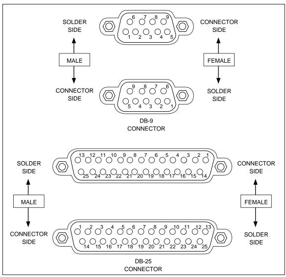
Figure F-6. RS-232 DB9 and DB-25 Connectors
