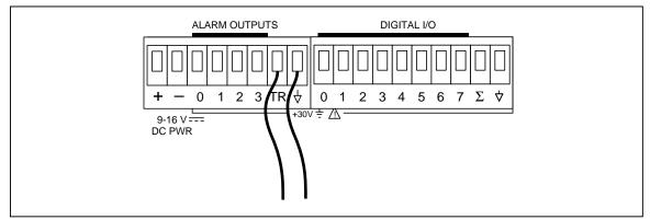
Figure 6-5. External Trigger Test
