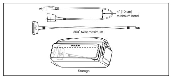
Figure 2-11. Permanent Link Adapter Handling Guidelines
