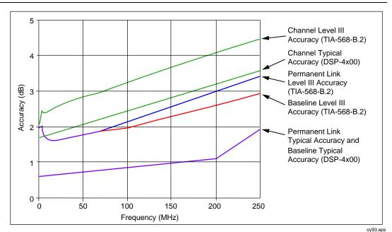
Figure 8-4. PSNEXT Measurement Accuracy for Channel
