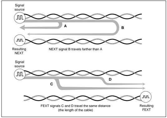
Figure 7-9. How FEXT Signals are All Equally Attenuated
