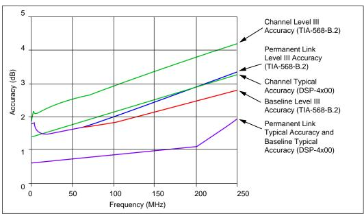
Figure 8-3. Pair-to-Pair NEXT Measurement Accuracy for a Channel
