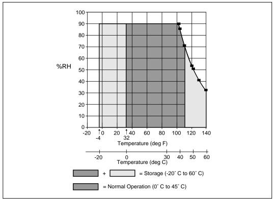
Figure 8-8. Operating Environment Specifications
