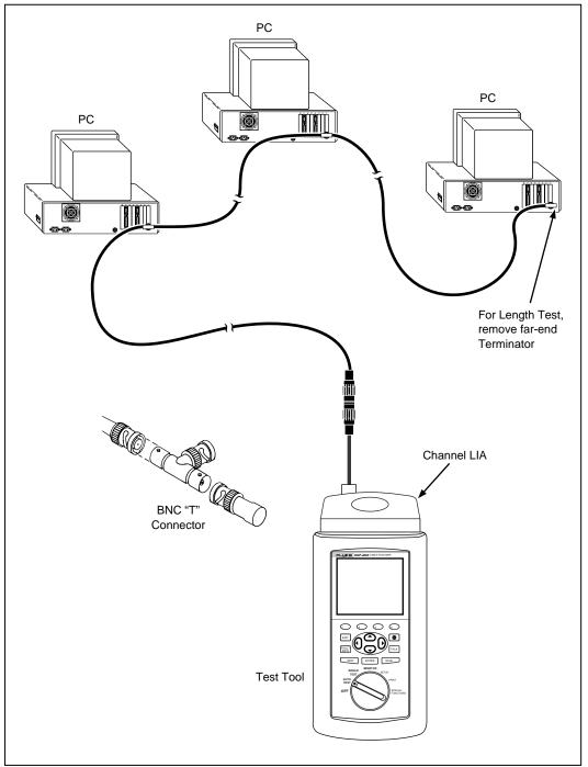
Figure 3-10. Autotest Connections for Coaxial Cabling
