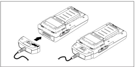
Figure 2-1. Attaching a Link Interface Adapter
