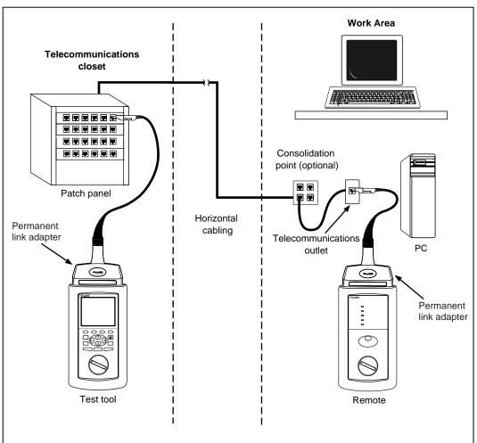
Figure 2-6. Typical Test Connections for a Permanent Link
