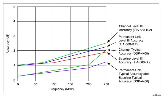
Figure 8-2. Attenuation (Insertion Loss) Measurement Accuracy for Channel
