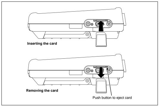
Figure 2-2. Inserting and Removing the Memory card
