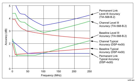
Figure 8-7. Return Loss Measurement Accuracy for Channel
