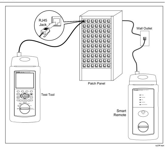
Figure 4-6. Typical Connections for Monitoring Impulse Noise
