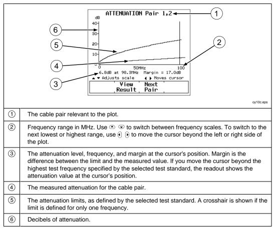
Figure 3-5. The Attenuation Plot Screen
