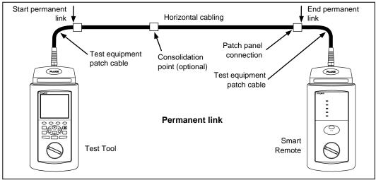
Figure 7-6. Permanent Link Test Connections
