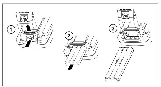
Figure 8-1. Removing the NiMH Battery Pack
