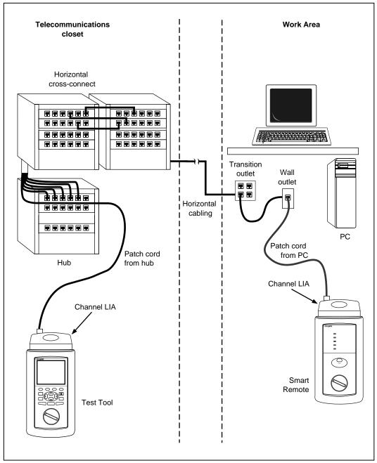
Figure 3-2. Typical Test Connections for a Channel
