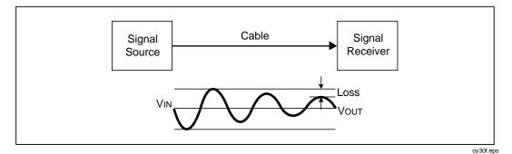
Figure 7-7. Attenuation of a Signal
