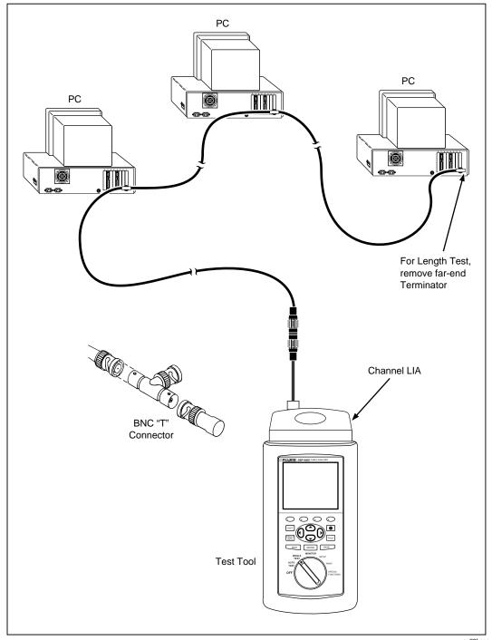
Figure 4-4. Single Test Connections for Coaxial Cabling
