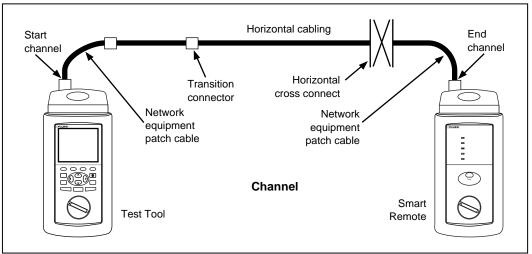
Figure 7-5. Channel Test Connections
