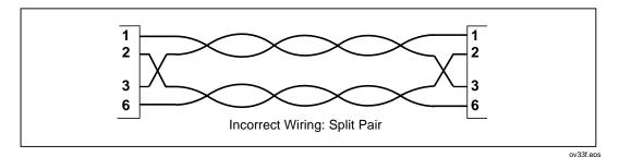
Figure 7-11. Split Pair Wiring
