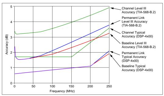
Figure 8-6. PSELFEXT Measurement Accuracy for Channel
