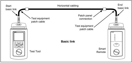
Figure 7-4. Basic Link Test Connections
