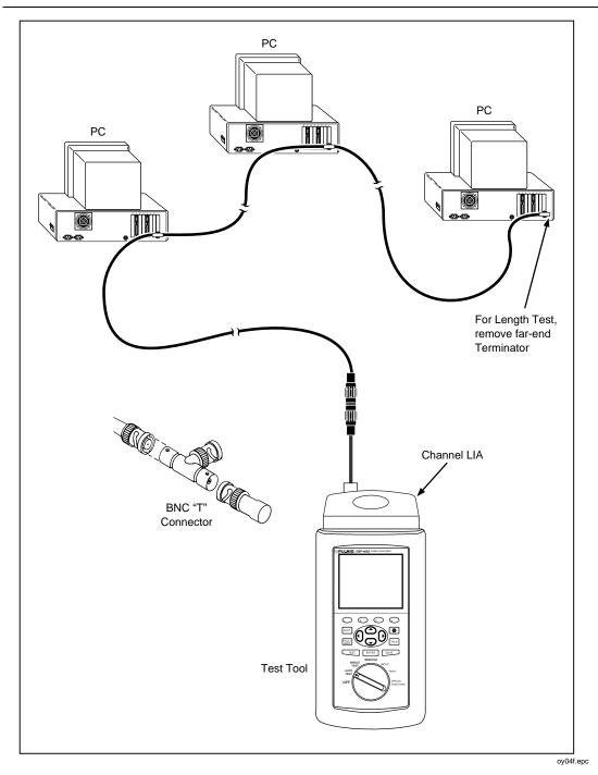
Figure 2-7. Autotest Connections for Coaxial Cabling
