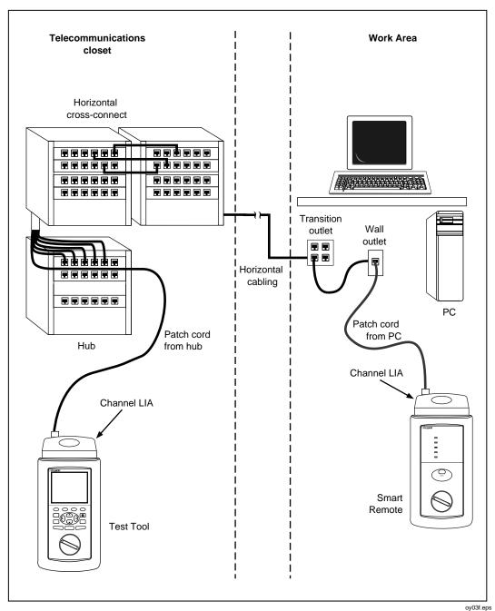
Figure 2-5. Typical Test Connections for a Channel
