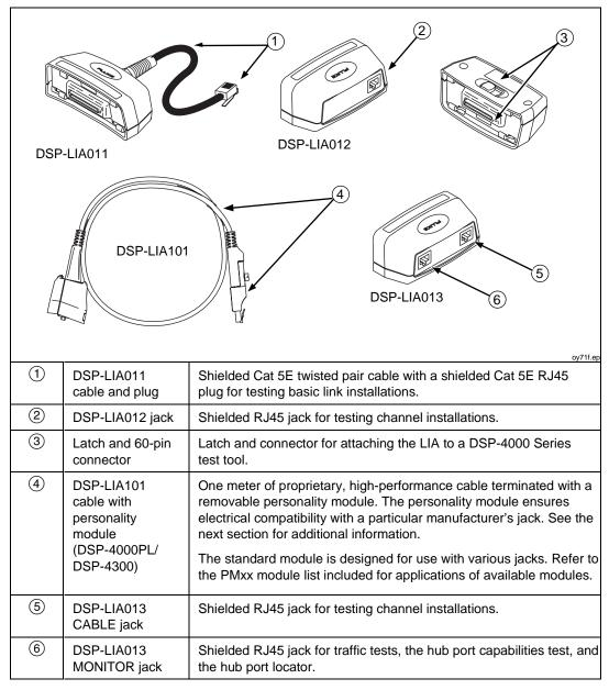
Figure 2-10. Link Interface Adapter Features
