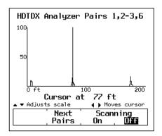
Figure 7-10. An HDTDX Analyzer Plot
