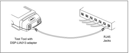
Figure 4-5. Connections for Monitoring Network Traffic
