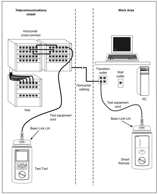
Figure 3-1. Typical Test Connections for a Basic Link
