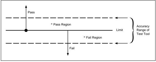
Figure 2-3. The Asterisk and Test Tool Accuracy
