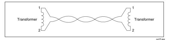
Figure 7-1. Twisted Pair Cable Construction
