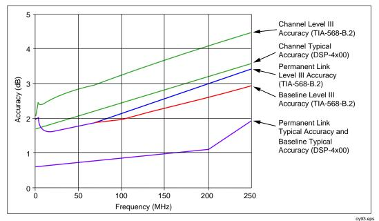
Figure 8-4. PSNEXT Measurement Accuracy for Channel
