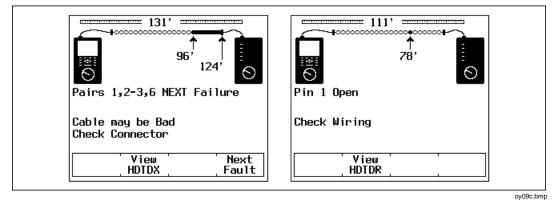
Figure 3-4. Examples of Automatic Diagnostics Displays
