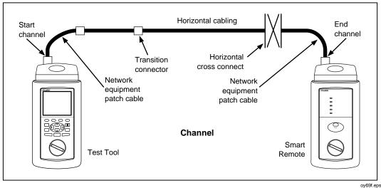
Figure 7-5. Channel Test Connections
