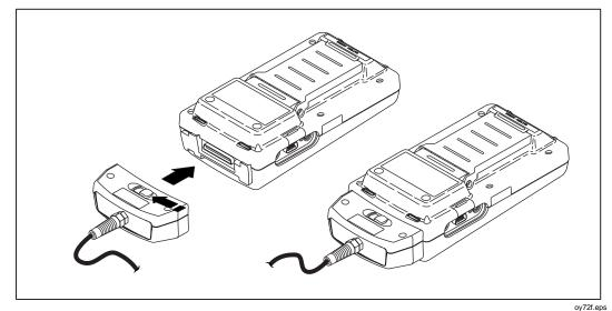
Figure 2-1. Attaching a Link Interface Adapter
