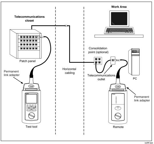
Figure 3-3. Typical Test Connections for a Permanent Link
