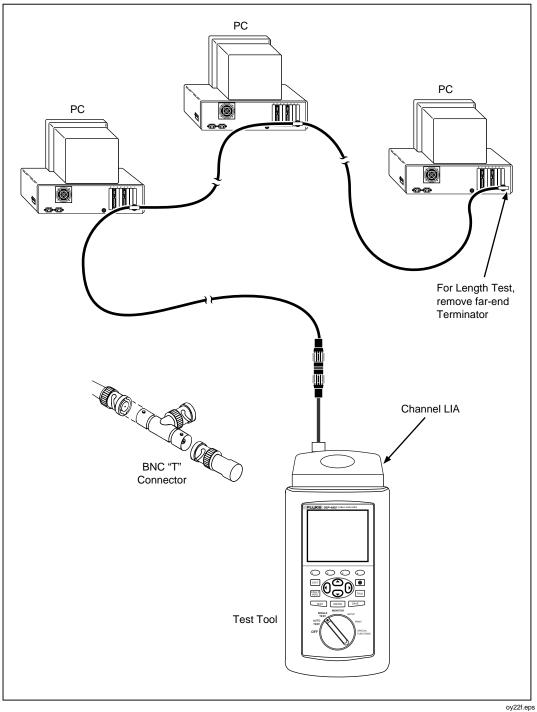
Figure 4-4. Single Test Connections for Coaxial Cabling
