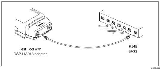
Figure 4-5. Connections for Monitoring Network Traffic
