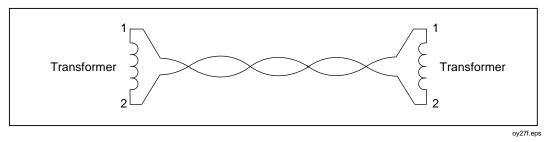
Figure 7-1. Twisted Pair Cable Construction
