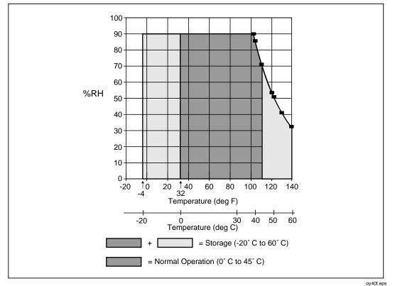
Figure 8-8. Operating Environment Specifications
