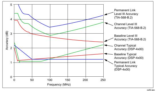
Figure 8-7. Return Loss Measurement Accuracy for Channel
