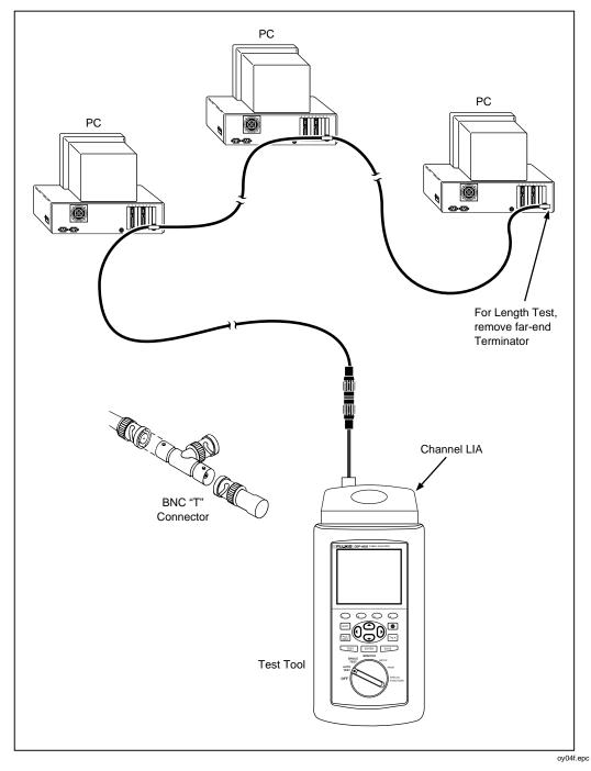
Figure 2-7. Autotest Connections for Coaxial Cabling
