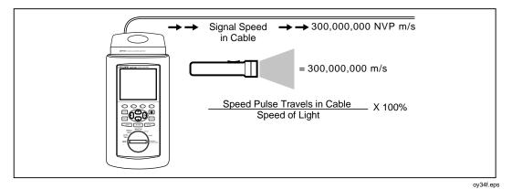
Figure 7-12. How NVP is Calculated
