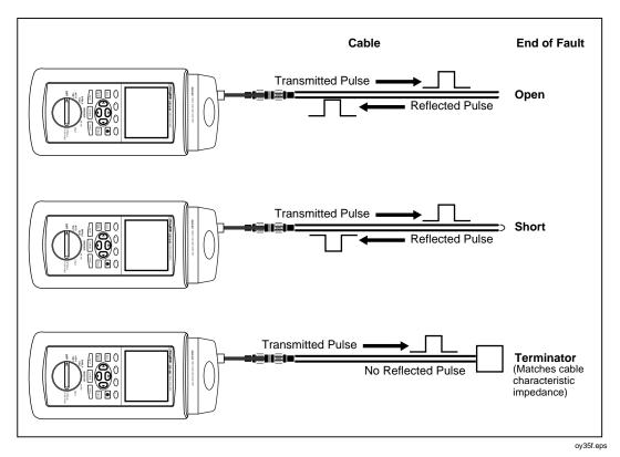
Figure 7-13. Signals Reflected from an Open, Shorted, and Terminated Cable
