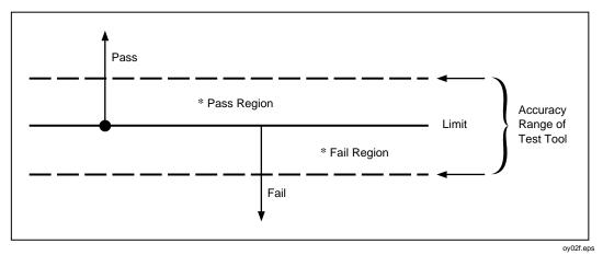
Figure 2-3. The Asterisk and Test Tool Accuracy
