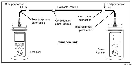
Figure 7-6. Permanent Link Test Connections
