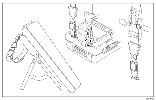
Figure 2-13. Attaching the Strap and Opening the Bail
