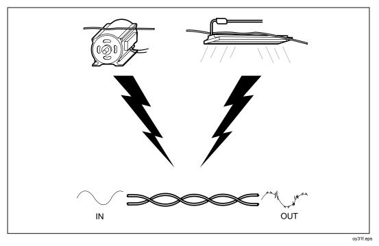
Figure 7-8. Sources of Electrical Noise
