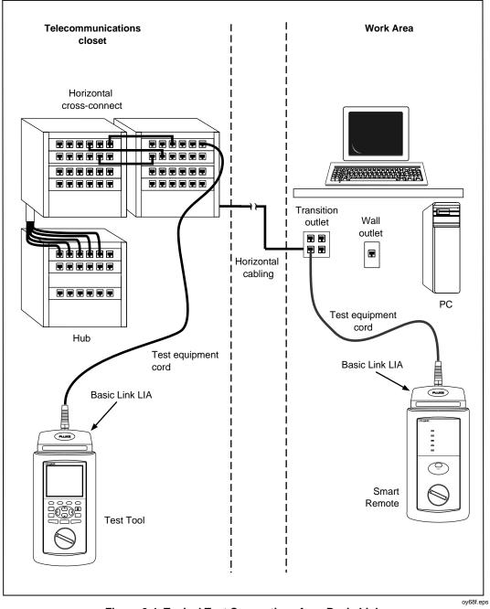
Figure 2-4. Typical Test Connections for a Basic Link
