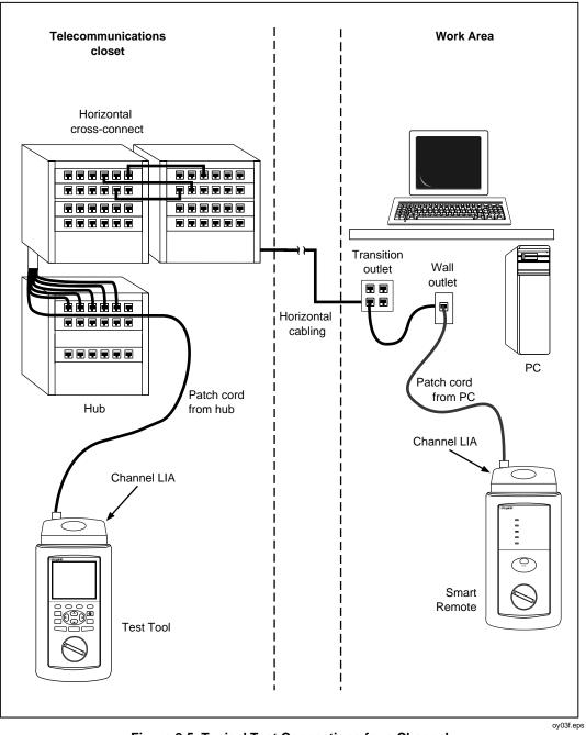
Figure 2-5. Typical Test Connections for a Channel
