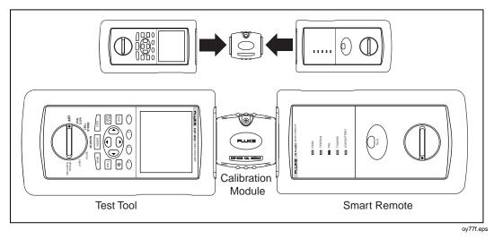
Figure 6-1. Connections for Self-Calibration
