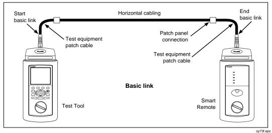
Figure 7-4. Basic Link Test Connections
