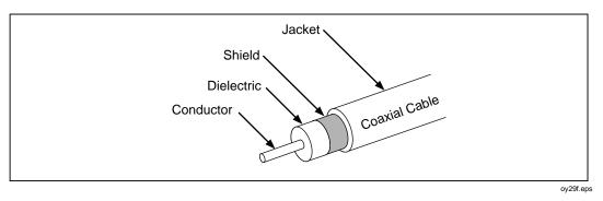
Figure 7-3. Coaxial Cable Construction
