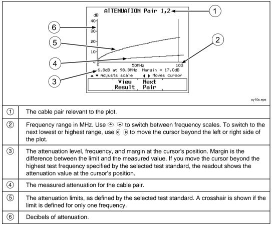
Pressing (a) View Plot produces the attenuation plot screen. Figure 3-5 describes an example of the screen.
