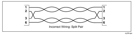
Figure 7-11. Split Pair Wiring
