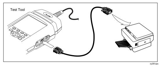
Figure 5-1. Connections for Printing Test Reports
