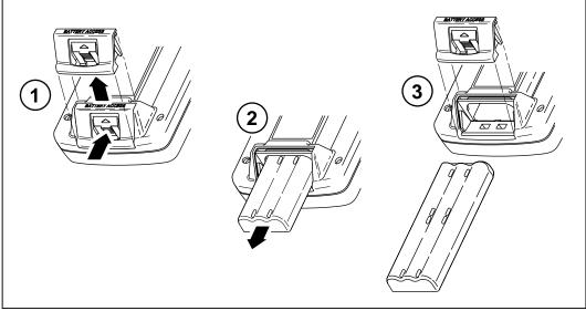
Figure 8-1. Removing the NiMH Battery Pack
