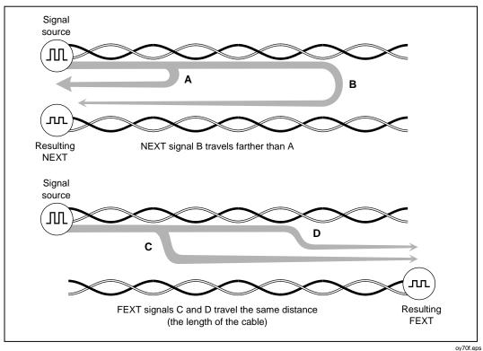
Figure 7-9. How FEXT Signals are All Equally Attenuated
