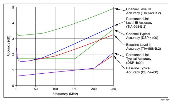
Figure 8-6. PSELFEXT Measurement Accuracy for Channel
