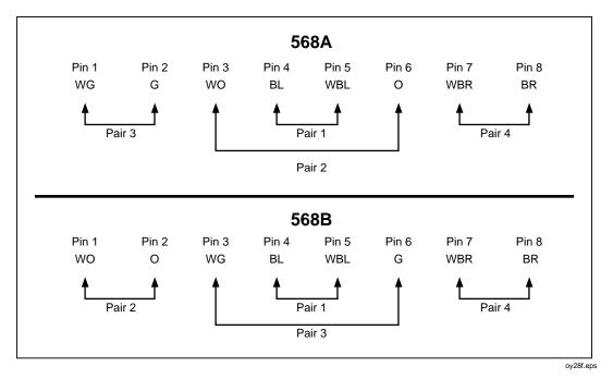
Figure 7-2 shows the pin connections and wire colors for correct wiring to TIA 568A and 568B standards.
