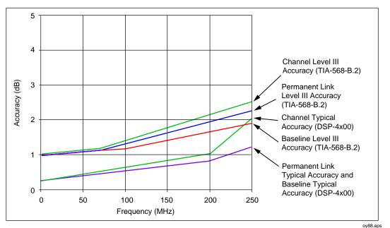
Figure 8-2. Attenuation (Insertion Loss) Measurement Accuracy for Channel
