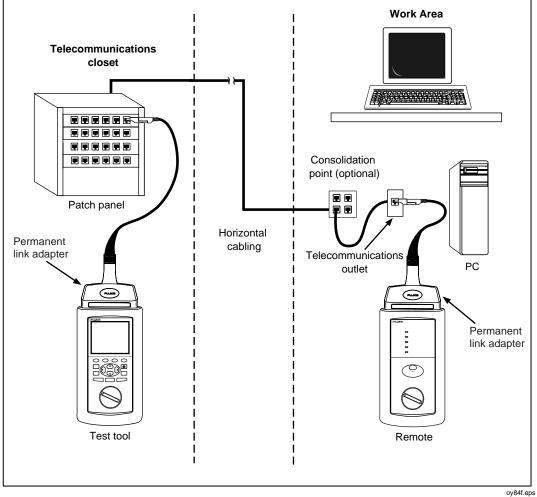
Figure 2-6. Typical Test Connections for a Permanent Link
