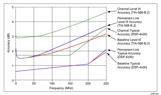
Figure 8-5. Pair-to-Pair ELFEXT Measurement Accuracy for Channel
