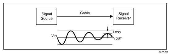
Figure 7-7. Attenuation of a Signal
