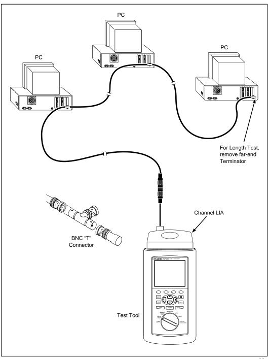
Figure 3-10. Autotest Connections for Coaxial Cabling
