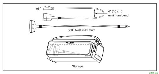
Figure 2-11. Permanent Link Adapter Handling Guidelines
