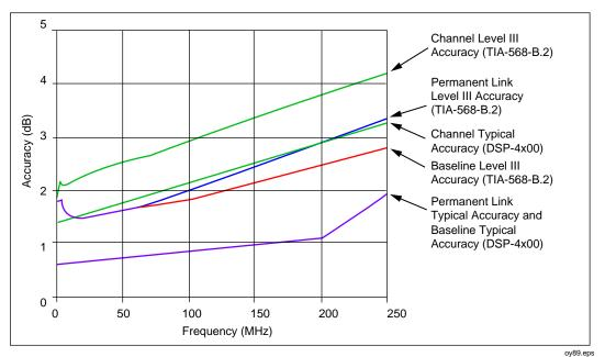
Figure 8-3. Pair-to-Pair NEXT Measurement Accuracy for a Channel
