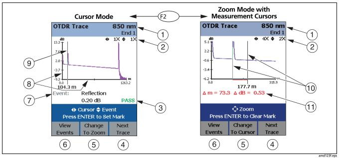
Figure 9. OTDR Trace Screens (launch compensation disabled)
