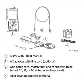
Figure 11. Equipment for Using the Visual Fault Locator
