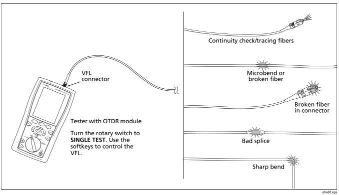
Figure 12. Using the Visual Fault Locator
