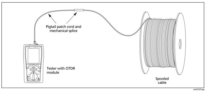
Figure 7. Connecting the OTDR to Spooled Cable
