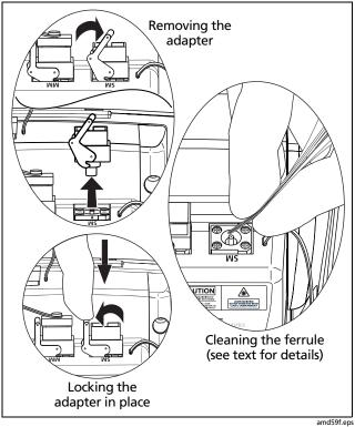
Figure 13. Cleaning the OTDR Ports
