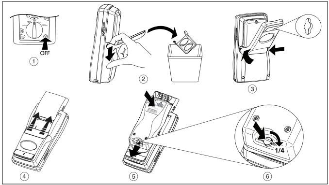
Figure 1. Installing the OTDR Module
