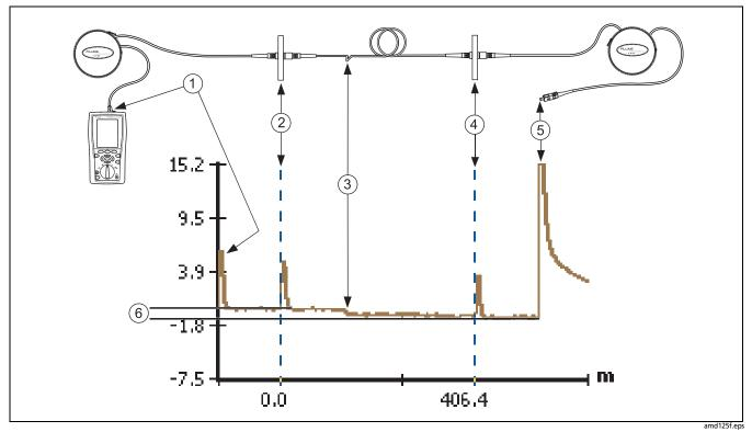
Figure 10. Typical OTDR Trace Features
