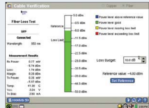
Ensure optical power limits are within specification
