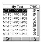
To view detailed information about a saved Autotest use the éê on your keypad to highlight a Circuit ID in the Project Name screen and press ENTER.
