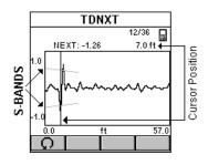
The NEXT at the cursor position relative to the S-Band, the corresponding pair combination, and the distance to the cursor position are displayed above the graph.
