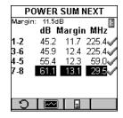
Press or to toggle between the PSNEXT results for OMNI-SCANNER and OMNIREMOTE.
