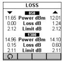
The **LOSS** screen displays the measured power in dBm (decibels; one milliwatt reference) for each wavelength.
