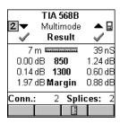
When dual fiber is measured, arrows st at the top of the screen point out the direction of the light. The arrows also indicate the fiber that the (PASS) or (FAIL) result is for.
