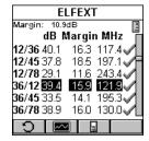
Press (Graph) to display the ELFEXT graph for the currently highlighted pair combination. ELFEXT is displayed for the frequency
