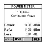
When testing loss, use the continuous light source, when identifying fiber cables with a tone locator, use the 2KHz modulated mode.
