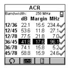
Bandwidth is a measure of the usable frequency range of the link under test. For most networks, this is the highest frequency at which the signal can easily be distinguished from background noise. Bandwidth is reported as the frequency where ACR is 3dB.
