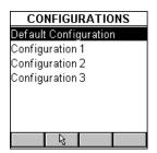
The predefined **Default Configuration** is always present and can be used to reset OMNISCANNER to the factory default. It contains the following projects: TIA, ISO/IEC, VENDOR, OMNI, IEEE, ATM, AS/NZ, ANSI.
