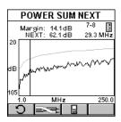
Press (Graph) to display the PSNEXT graph for the currently highlighted pair. PSNEXT is displayed for the frequency indicated by the cursor position.
