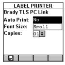
Press ENTER to turn the **Auto Print** feature on or off. Select **YES** if you want OMNISCANNER to automatically print a label after the Autotest has been saved. Select **NO** if you want to manually initiate the print process. Press ENTER when done.
