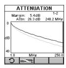
Press (Graph) to display the Attenuation graph for the highlighted pair. The Attenuation is displayed for the frequency indicated by the cursor position.
