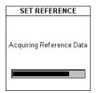
Connect OMNISCANNER and OMNIREMOTE through their test connector ports using the Link Adapter and the Channel Adapter. Select **Set Reference** to display the **SET REFERENCE** screen.
