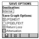
Press (Save to MMC) to save the test results to the MultiMediaCard. (OMNIScanner2 only.)
