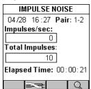
Select Impulse Noise to open the **IMPULSE NOISE** screen. The current date and time is shown in the upper left. The monitored pair is shown in the upper right.
