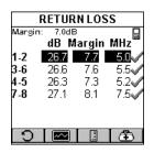
The pairs are displayed in the column on the left side, followed by the Return Loss in decibels (dB), the Return Loss margin/limit, and the frequency. The result for each pair is tagged with a PASS , Marginal PASS , Marginal FAIL , or FAIL , indicator.
