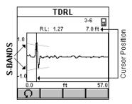
Initially, the cursor is located at the point with the worst Return Loss.
