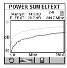
Press (Graph) to display the PSELFEXT graph for the currently highlighted pair. PSELFEXT is displayed for the frequency indicated by the cursor position.
