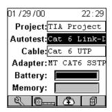
Battery and Memory status are graphically indicated by gauges with a display ranging from empty (left hand side) to full (right hand side).
