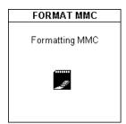
To format the MultiMediaCard, select **Format MMC** in the **SETUP** screen. A gauge will indicate the progress. (See Chapter 4 - Setup: **Format MMC** for further information.)
