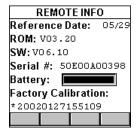
The **Battery** status is represented with a gauge. **Factory Calibration\*** data is displayed at the bottom of the screen.
