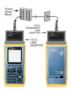
LINK ADAPTER to attach OMNIREMOTE to the Modular 8 jack.
