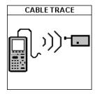
1. Attach the end of the cable you want to trace to the OMNISCANNER using a patch cord and the Channel Adapter or the Link Adapter. Make sure that the cable is not grounded, as a grounded cable will weaken the signal.
