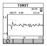
NEXT in the cable is the source of the failure even though the cable's NEXT response peaks are less than those of the connection. By knowing that the connection meets its performance requirement, the cable is easily identified as the non-compliant component of the link.
