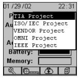
The Project feature is very useful for grouping test results and eases uploading and sorting of Autotests stored in the scanner.
