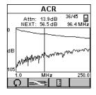
Press (Graph) to view the graph for the currently highlighted pair combination. The values for Attenuation and NEXT are shown at the top of the screen. Attenuation and NEXT graphs are displayed for the frequency indicated by the cursor position.
