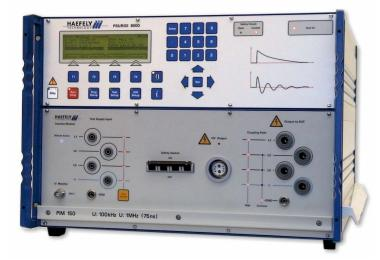
The modular concept is built around a PC based host controller (the PSURGE 8000 Controller) with physically and functionally independent modules for impulses (PIM #X), coupling/decoupling (PCD #X). The system uses distributed intelligence, and each module has its own application-specific program, runs internal routines and communicates with the host controller. System modules are automatically detected by the host controller, providing true Plug & Play functionality.
