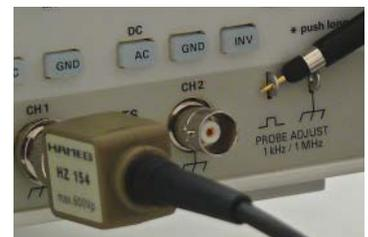
probe manual for its location) until the square wave is perfectly flat, i.e. there are neither under- nor overshoots. The transitions are invisible at this sweep speed (see the pictures). The amplitude of the square wave should be within  $4 \pm 0.12$  DIV.
