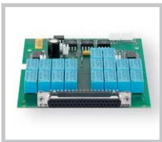
HM8112-3X: Multimeter with built-in Scanner Card (8+1 channels, 4 wire)
