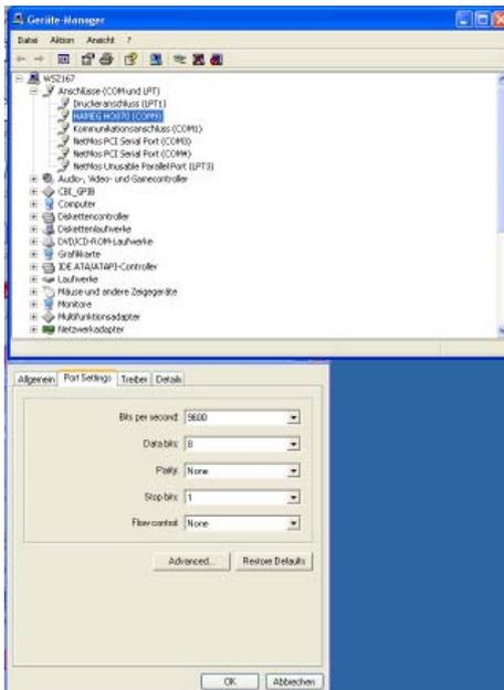
9. After successful installation the “Found New Hardware Wizard” opens again, in order to install the USB Serial Port. Proceed as described under the points 1 to 8. After the installation is complete, you can see the virtual COM Port in your Windows Device Manager. Set the COM port settings according to the transmission data of the measuring instrument (see manual of the instrument).
