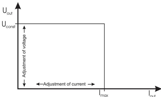
The picture shows that the output voltage  $V_{out}$  remains stable, while the current  $I_{out}$  increases until the current limit selected  $I_{max}$  will be reached. At this moment the instrument will change from constant voltage regulation to constant current regulation. Any further load increase will cause the current to remain stable while the voltage  $U_{out}$  decreases ultimately to zero.
