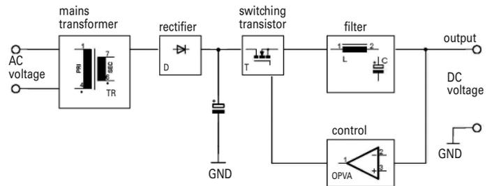
small due to the high frequency, but the choice depends also on other factors like energy required for buffering or ac ripple from the load (e.g. motors). In principle the size of the major components decreases with increasing operating frequency, however, the efficiency drops appreciably above appr. 250 kHz as the losses in all components rise sharply.
