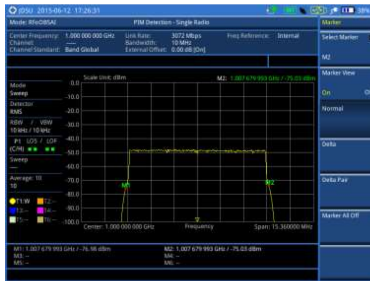
Figure 399 PIM detection of single radio
