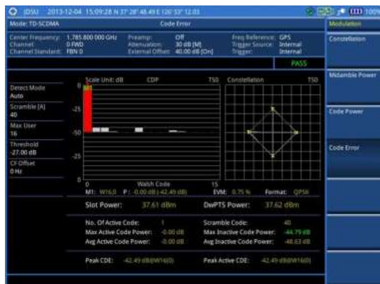
Figure 271 Code error measurement with TD-SCDMA signal analyzer
