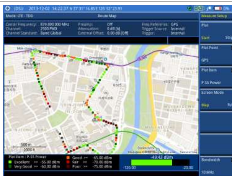
Figure 199 Route map measurement (P-SS Power) with LTE-TDD OTA signal analyzer
