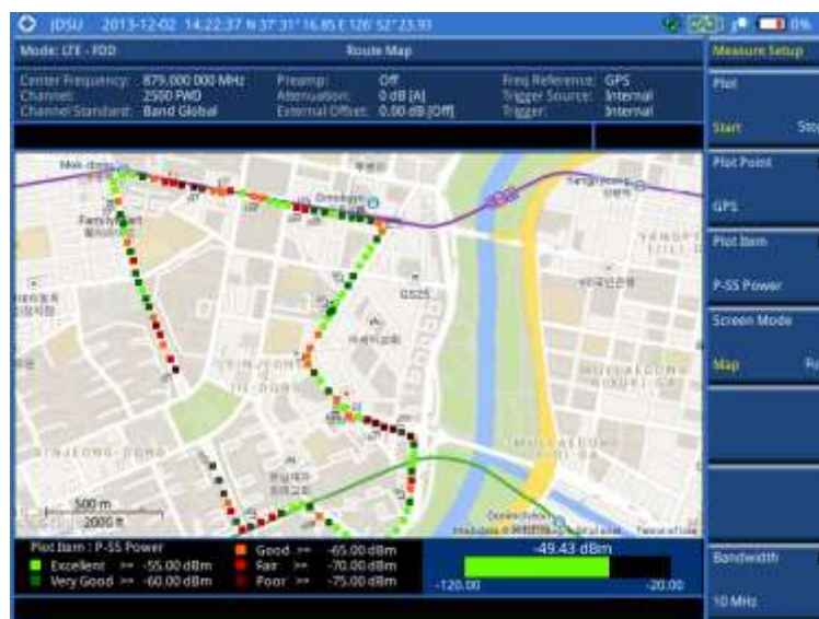
Figure 154 Route map measurement (P-SS Power) with LTE-FDD OTA signal analyzer
