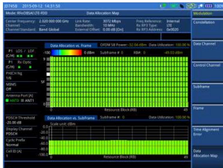
Figure 412 Data allocation map measurement with RFoOBSAI LTE-FDD signal analyzer
