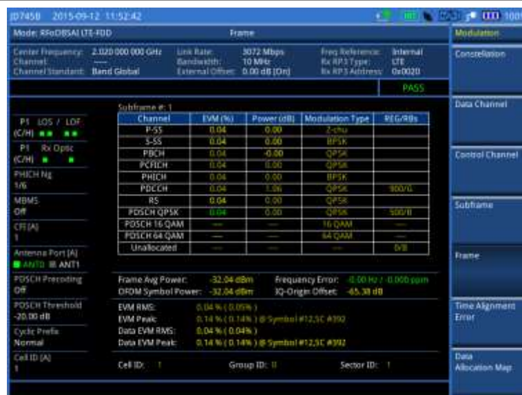
Figure 410 Frame measurement with RFoBSAI LTE-FDD signal analyzer
