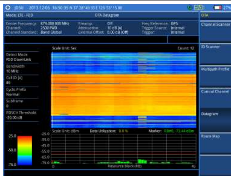
Figure 149 Datagram measurement with LTE-FDD signal analyzer
