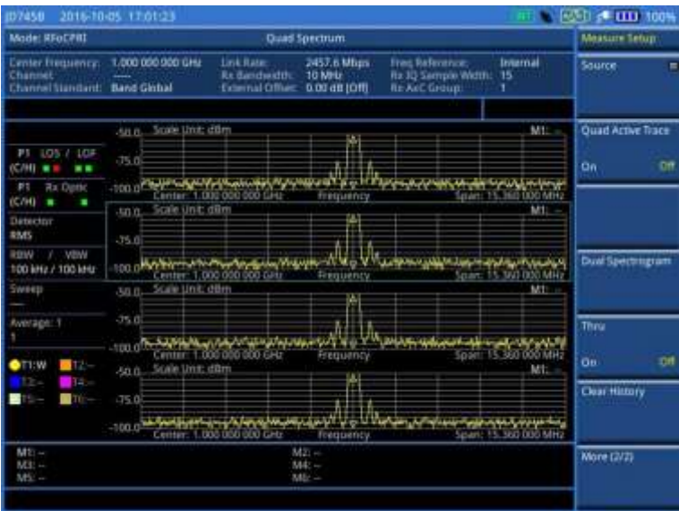
Figure 354 RFoCPRI quad spectrum with quad active trace on
