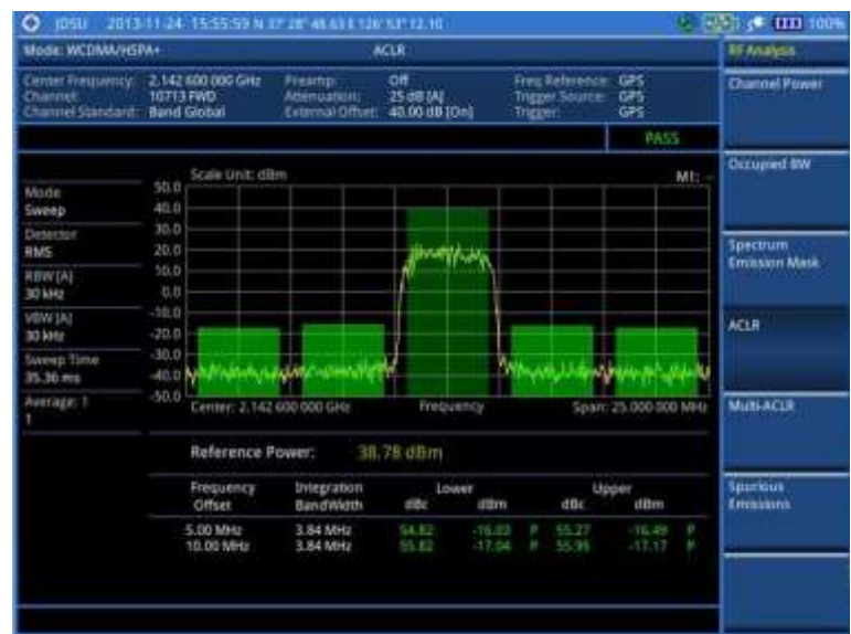
Figure 93 ACLR measurement with WCDMA/HSPA+ signal analyzer
