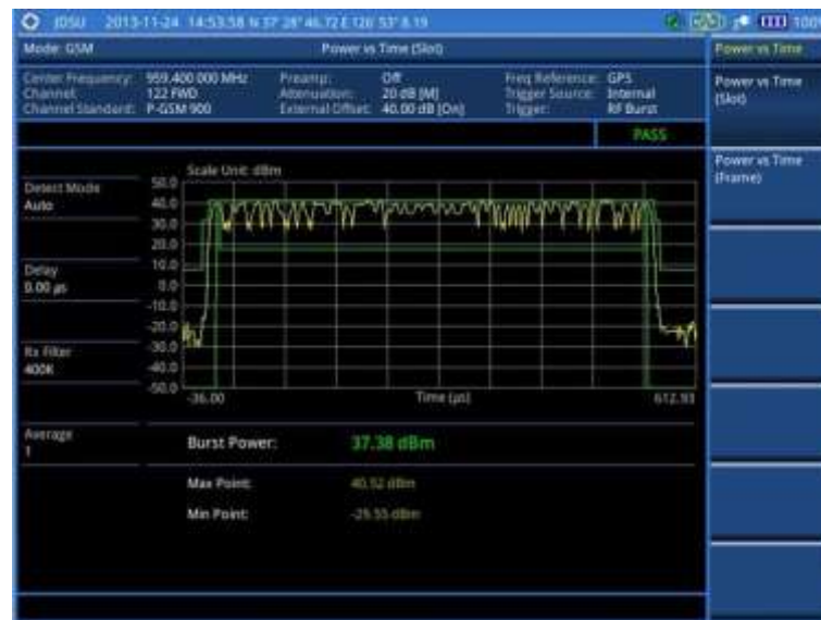
Figure 76 Power vs. time (slot) measurement with GSM signal analyzer
