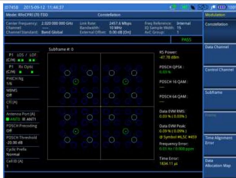
Figure 381 Constellation measurement with RFoCPRI LTE-TDD signal analyzer
