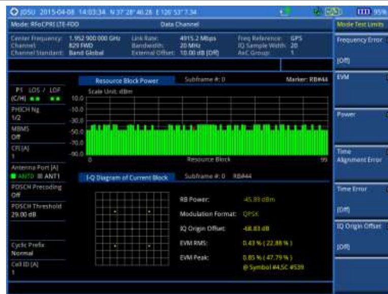
Figure 368 Data channel measurement with RFoCPRI LTE-FDD signal analyzer
