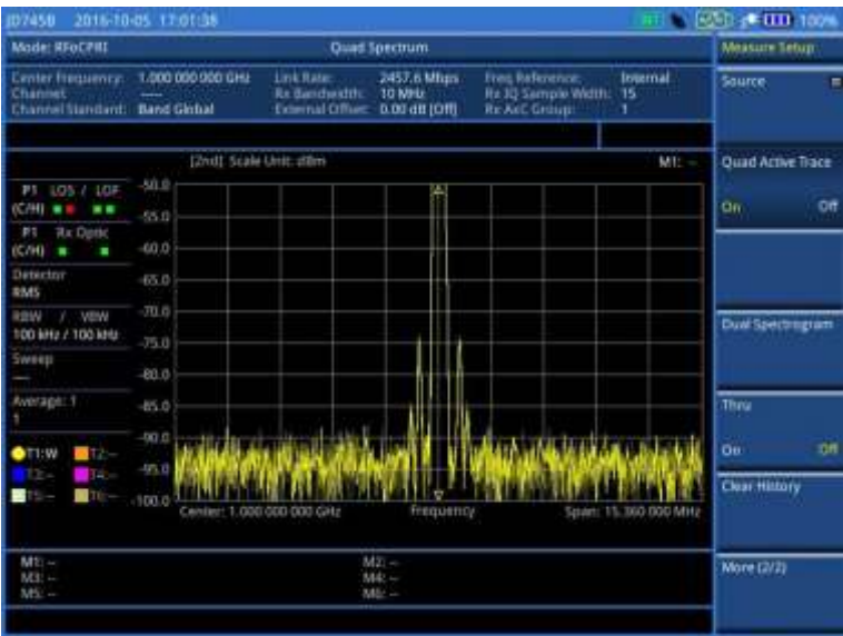
Figure 354 RFoCPRI quad spectrum with quad active trace on
