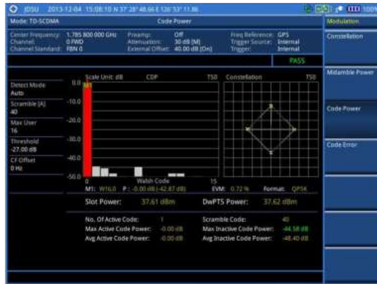
Figure 270 Code power measurement with TD-SCDMA signal analyzer
