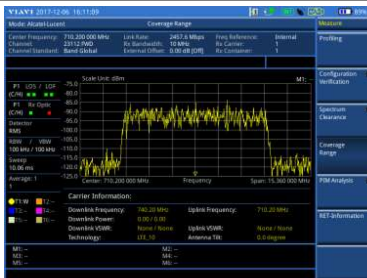
Figure 432 Example of coverage range in Alcatel-Lucent BBU emulation
