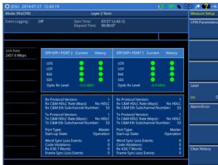
Figure 338 CPRI layer 2 term test
