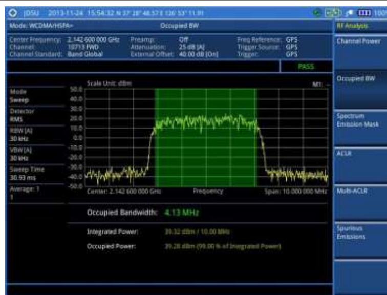
Figure 91 Occupied bandwidth measurement with WCDMA/HSPA+ signal analyzer
