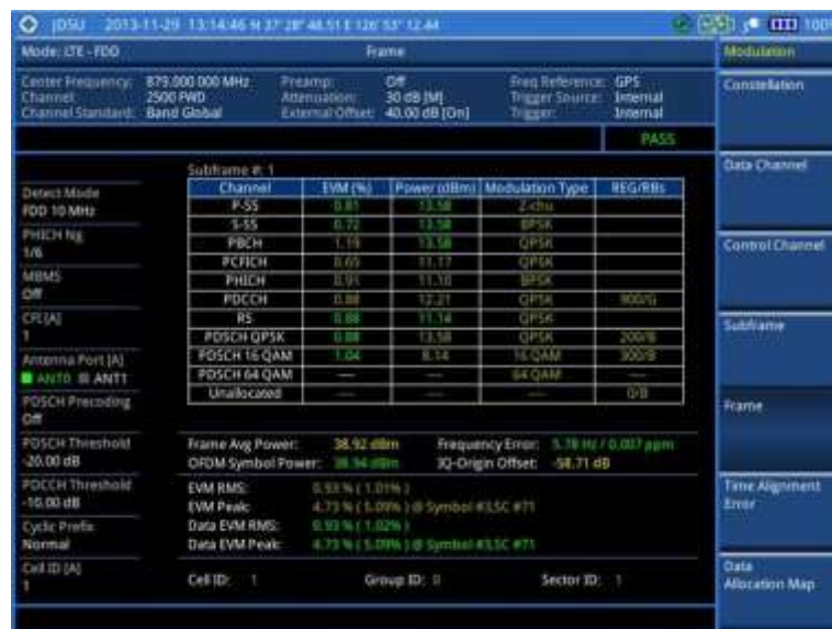
Figure 133 Frame measurement with LTE-FDD signal analyzer
