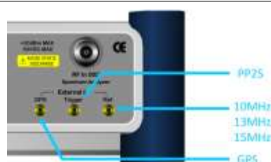
Figure 163 Connection ports for external reference clock
