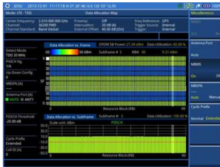
Figure 184 Data allocation map measurement with LTE-TDD signal analyzer (MBMS On)
