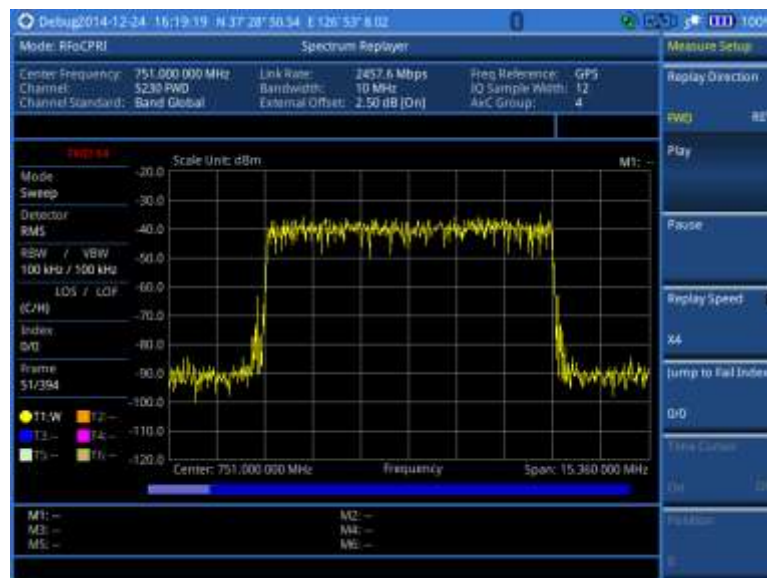
Figure 359 RFoCPRI spectrum replay
