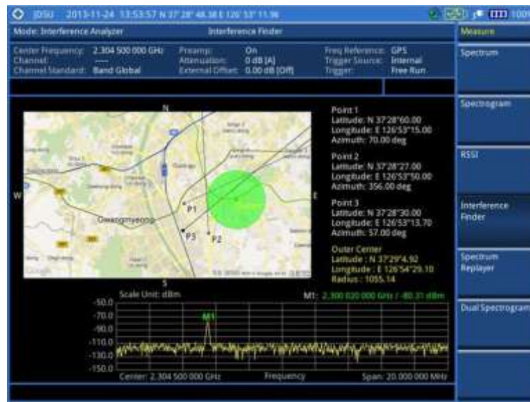
Figure 58 Interference finder measurement in map view (on 28 GHz downconverter)
