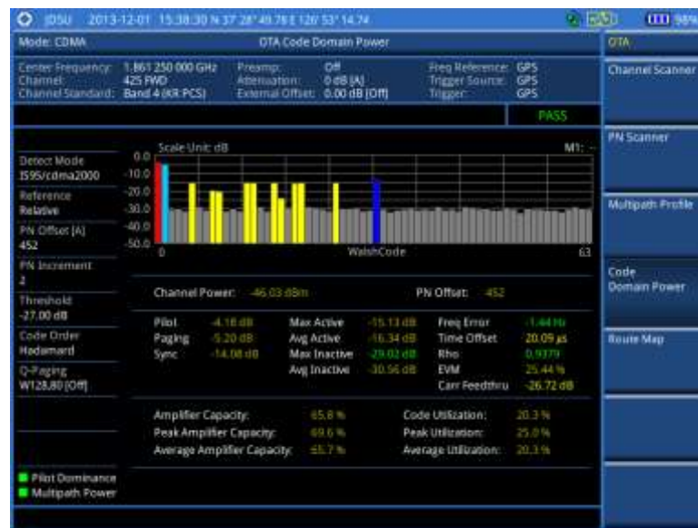
Figure 225 Code domain power measurement with CDMA OTA signal analyzer
