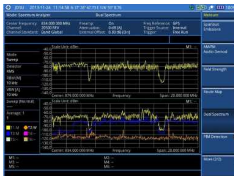
Figure 42 Dual spectrum measurement with spectrum analyzer
