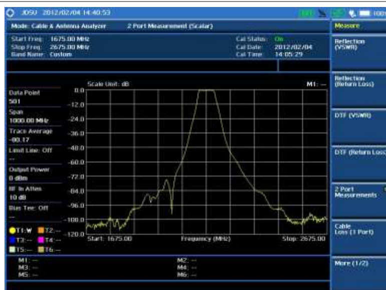
Figure 333 2-port scalar measurement
