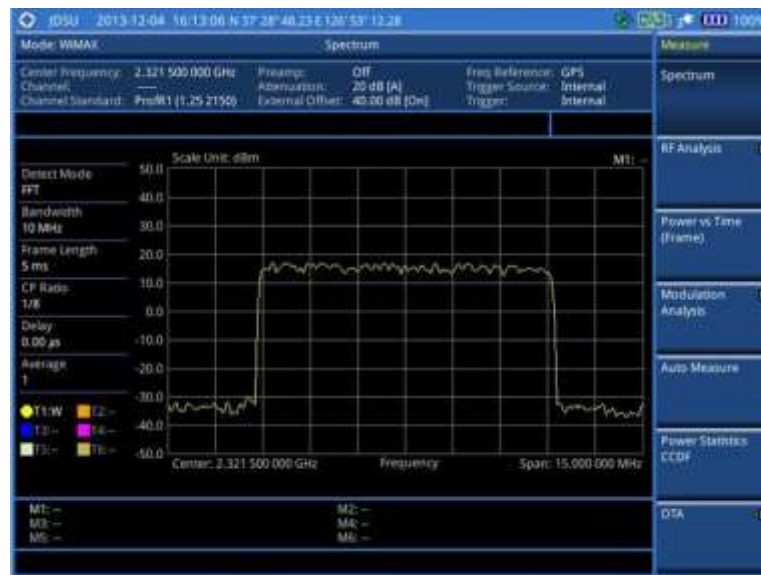
Figure 282 Spectrum measurement screen with Mobile WiMAX signal analyzer
