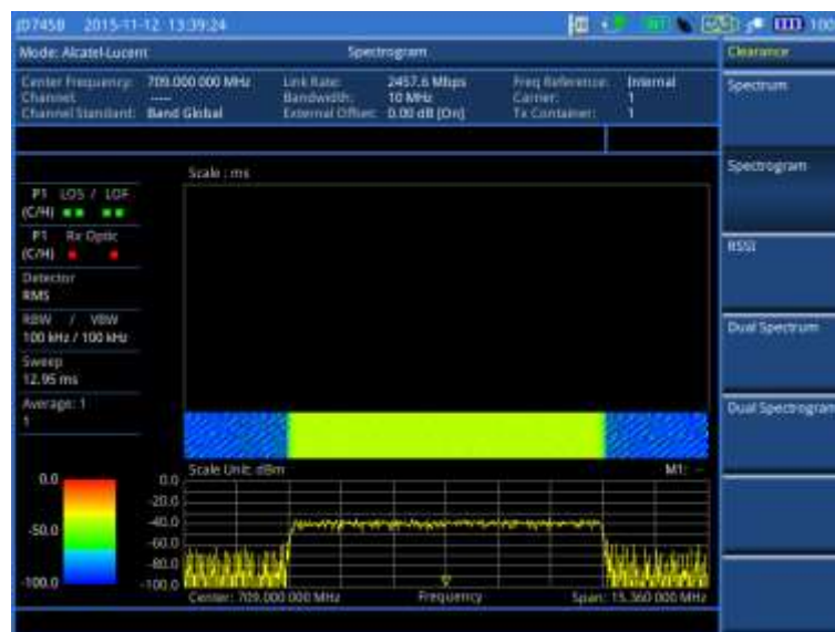
Figure 429 Example of spectrogram in Alcatel-Lucent BBU emulation
