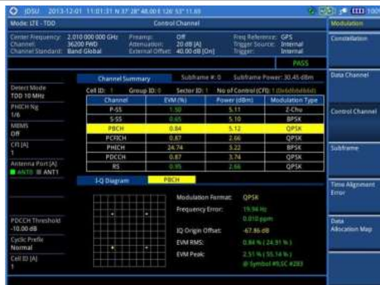
Figure 177 Control channel measurement with LTE-TDD signal analyzer
