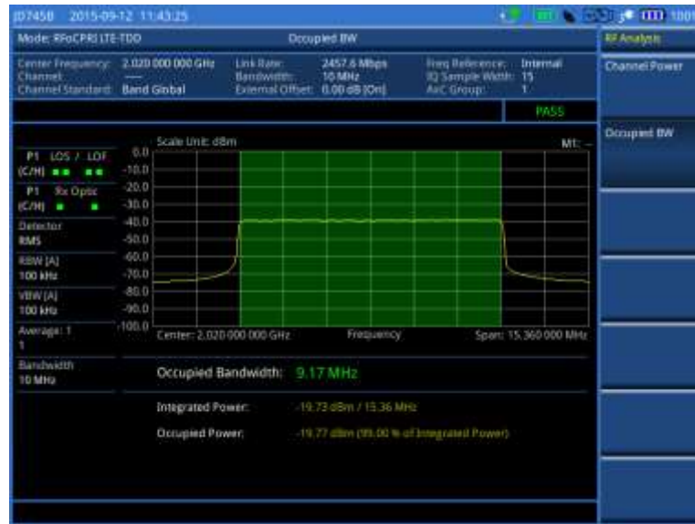
Figure 379 Occupied bandwidth measurement with RFoCPRI LTE-TDD signal analyzer
