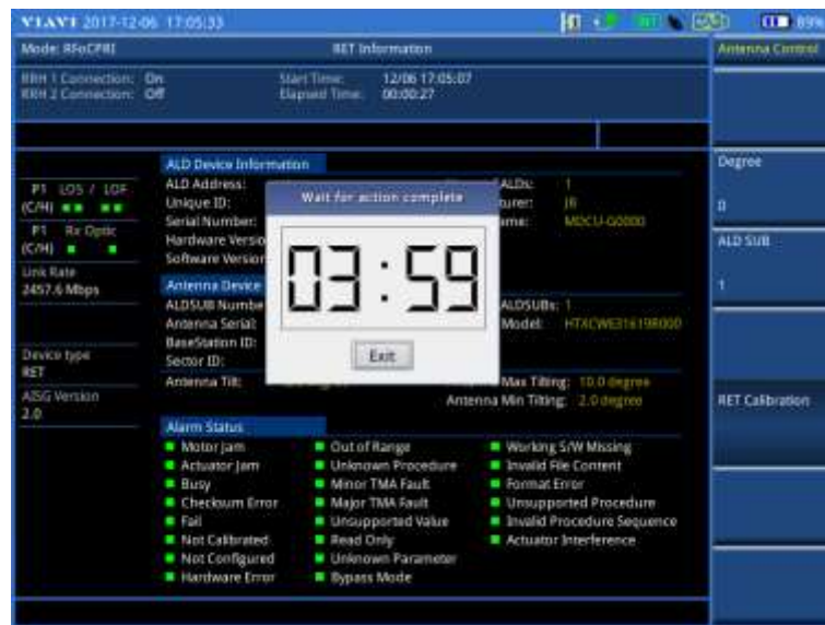
Figure 440 Example of RET calibration in Alcatel-Lucent RET information
