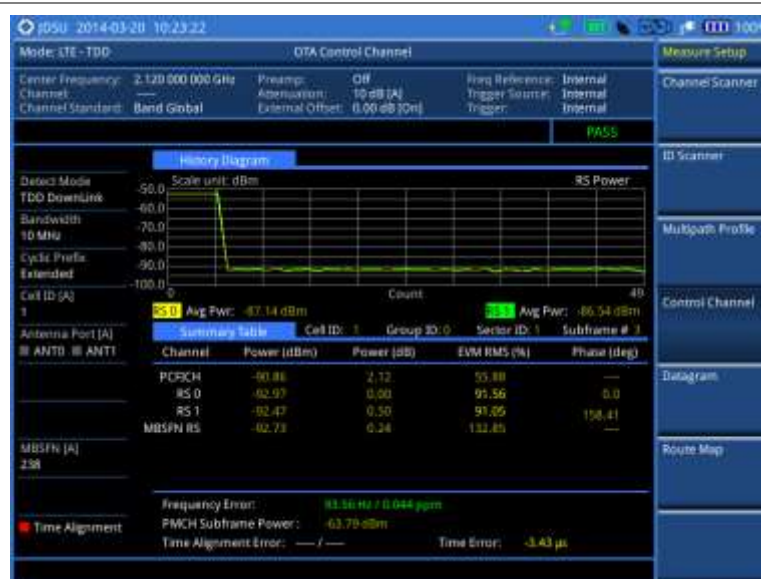
Figure 193 Control channel measurement with LTE-TDD OTA signal analyzer
