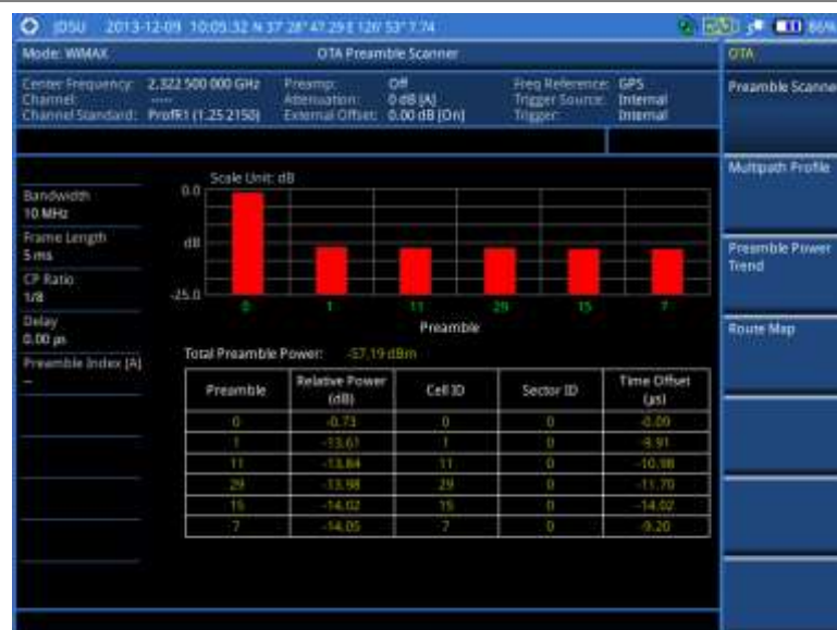
Figure 293 Preamble scanner measurement with Mobile WiMAX OTA signal analyzer
