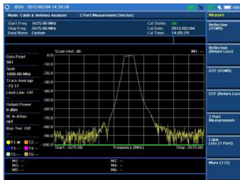
Figure 332 2-port vector measurement
