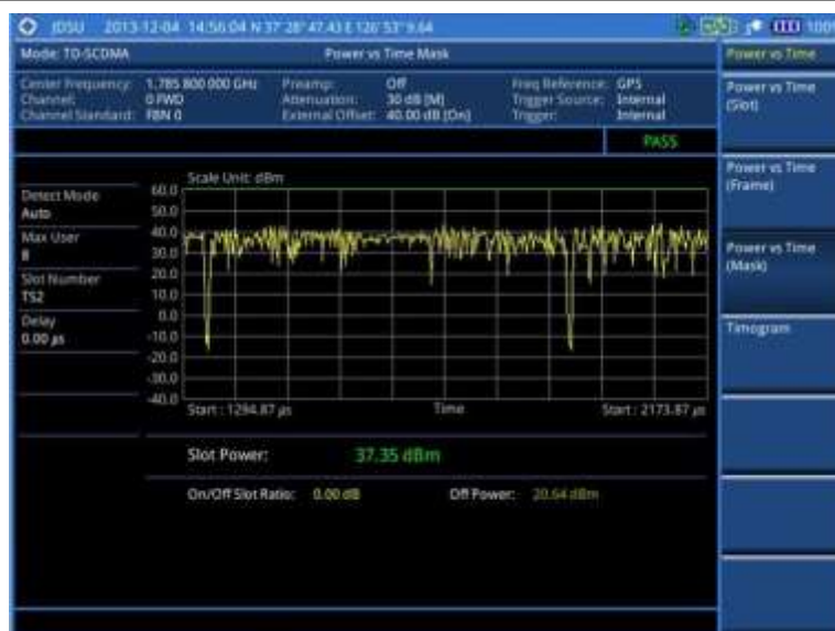
Figure 266 Power vs. time (mask) measurement with TD-SCDMA signal analyzer
