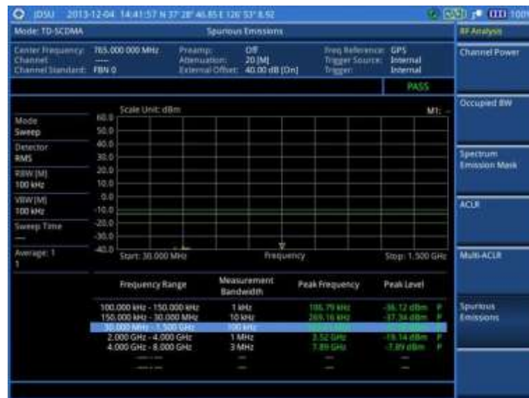
Figure 263 Spurious emissions measurement with TD-SCDMA signal analyzer
