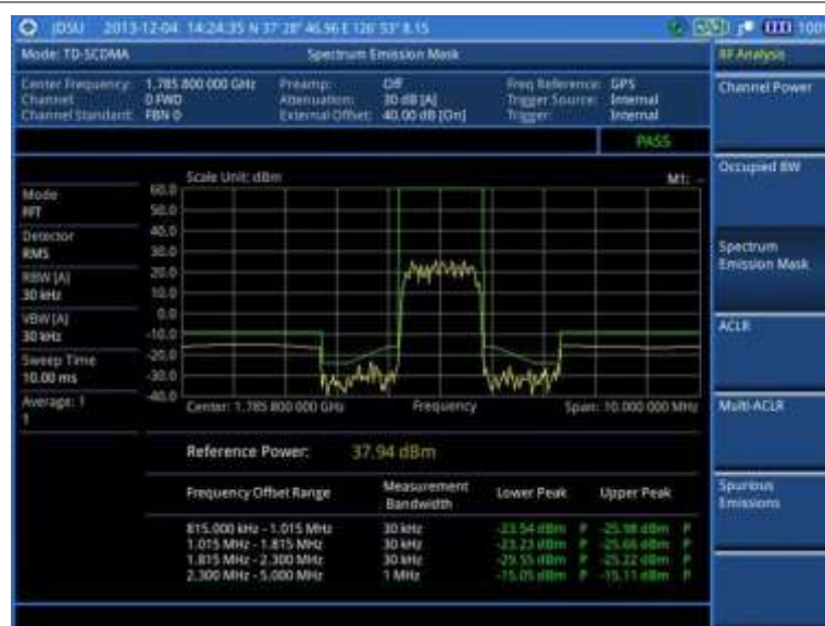
Figure 260 SEM measurement with TD-SCDMA signal analyzer
