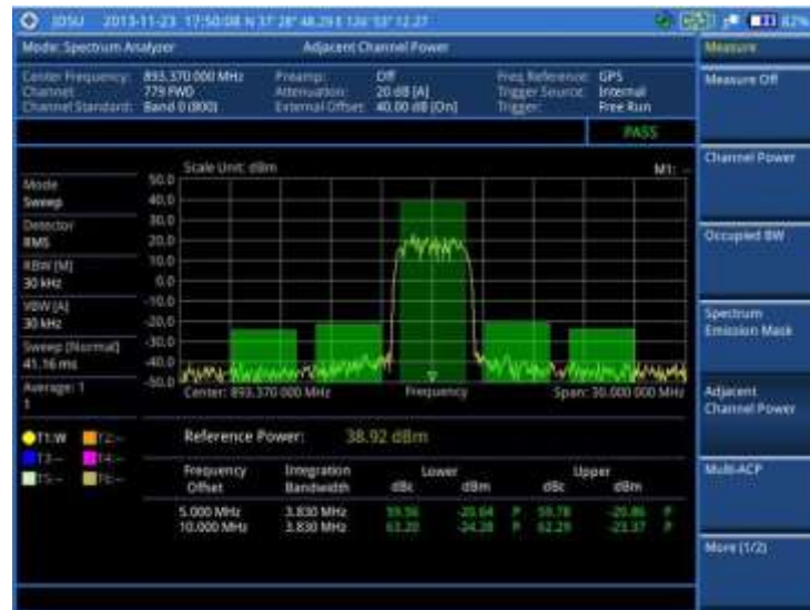
Figure 31 Adjacent channel power measurement with spectrum analyzer (on 28 GHz downconverter)
