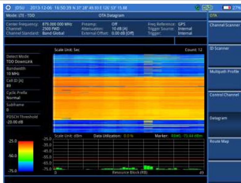
Figure 194 Datagram measurement with LTE-TDD signal analyzer
