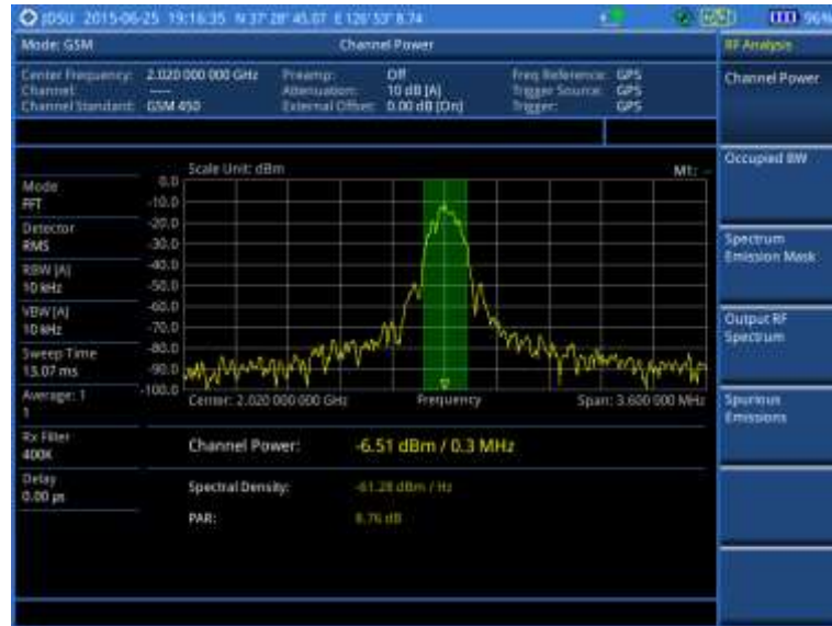
Figure 70 Channel power measurement with GSM signal analyzer
