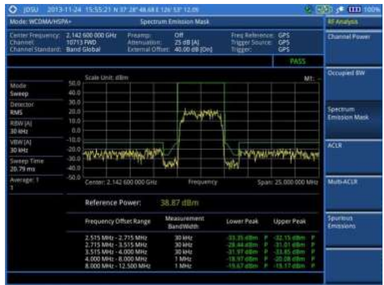
Figure 92 SEM measurement with WCDMA/HSPA+ signal analyzer
