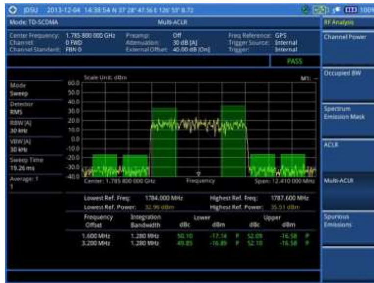
Figure 262 Multi-ACLR measurement with TD-SCDMA signal analyzer
