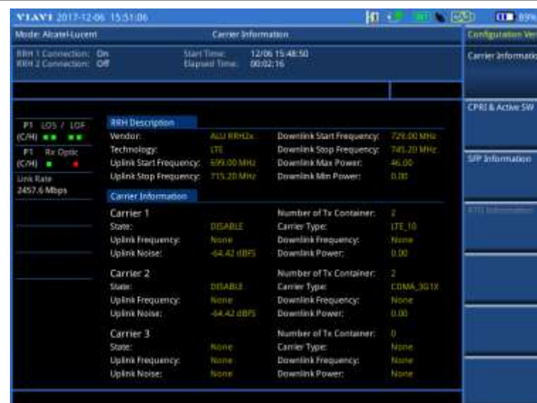
Figure 421 Example of verification of carrier configuration
