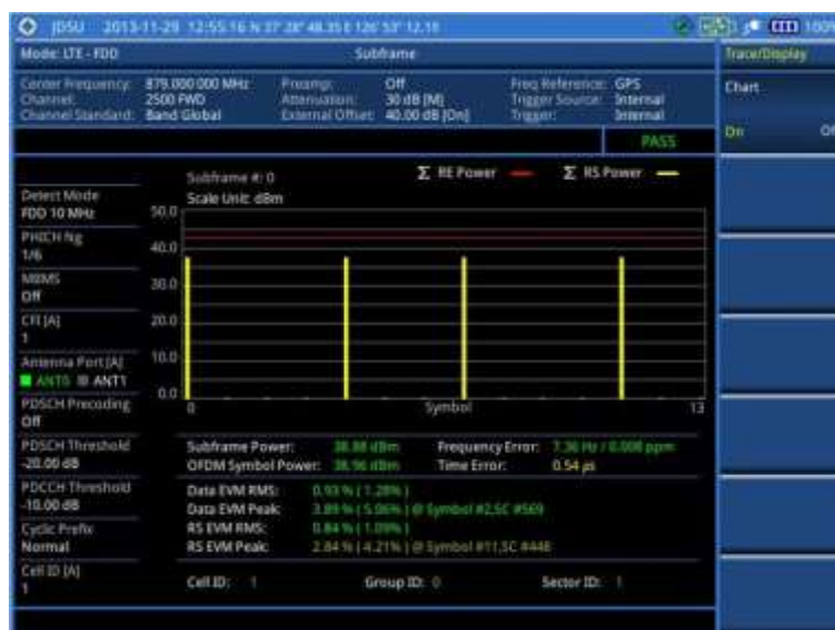
Figure 131 Subframe measurement with LTE-FDD signal analyzer (Chart On)
