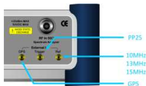
Figure 231 Connection ports for external reference clock
