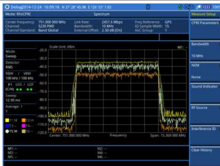
Figure 349 RFoCPRI spectrum analysis on LTE Uplink 10 MHz, antenna 2
