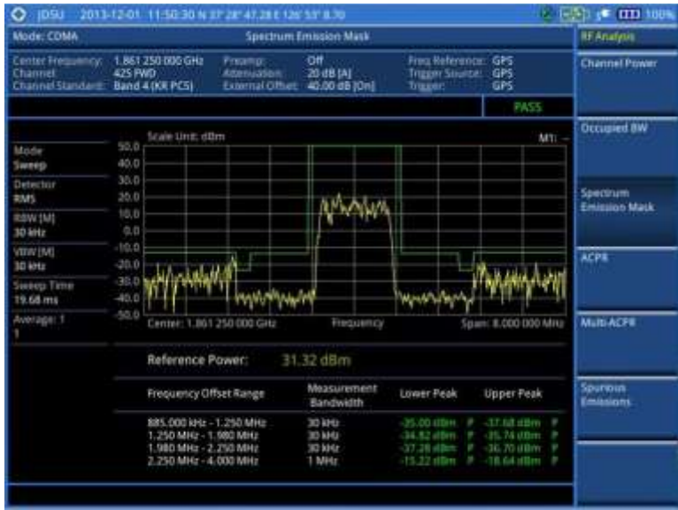
Figure 212 SEM measurement with CDMA signal analyzer
