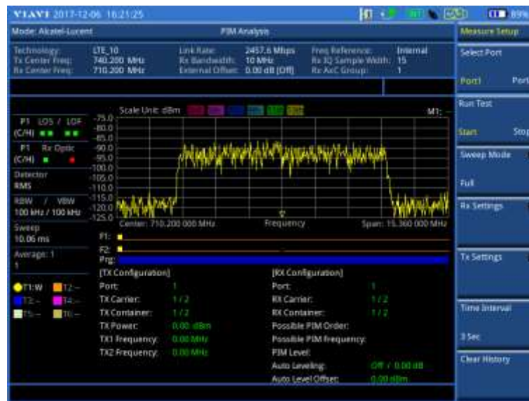
Figure 433 Example of single port sweep mode PIM Analysis in Alcatel-Lucent BBU emulation
