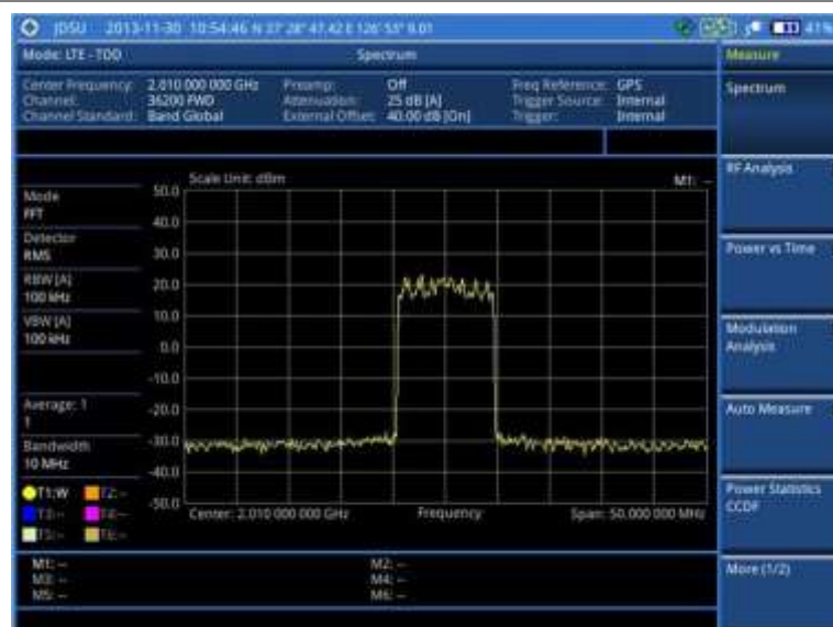
Figure 164 Spectrum measurement screen with LTE-TDD signal analyzer
