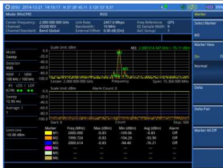
Figure 357 RFoCPRI interference measurement in RSSI
