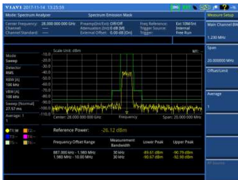
Figure 29 Spectrum emission mask measurement with spectrum analyzer (on 28 GHz downconverter)
