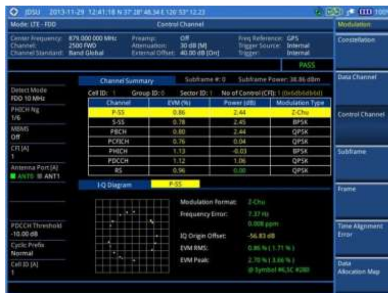
Figure 128 Control channel measurement with LTE-FDD signal analyzer
