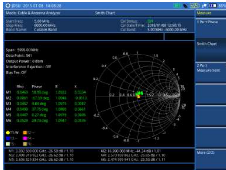
Figure 331 Smith chart measurement
