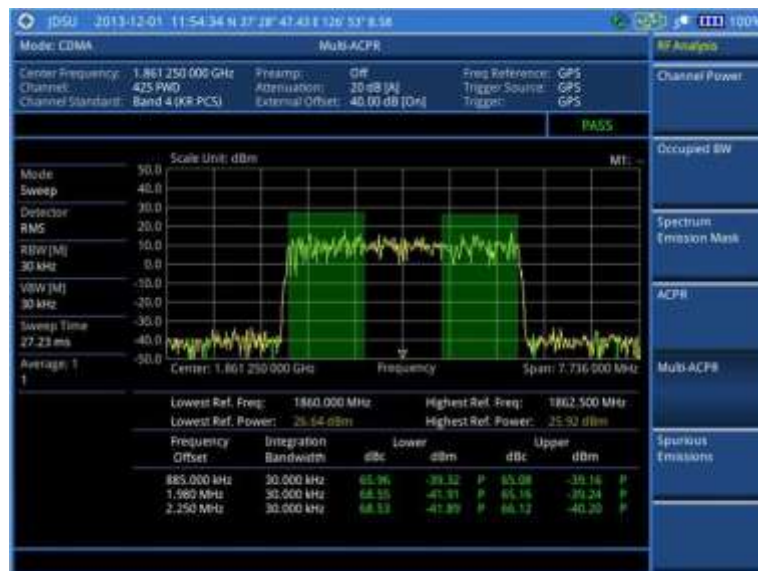
Figure 214 Multi-ACPR measurement with CDMA signal analyzer
