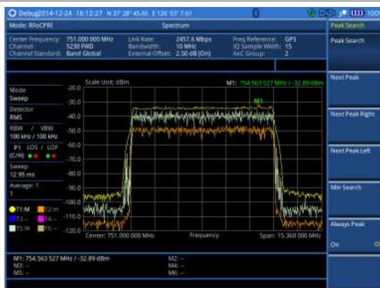
Figure 349 RFoCPRI spectrum analysis on LTE Uplink 10 MHz, antenna 2
