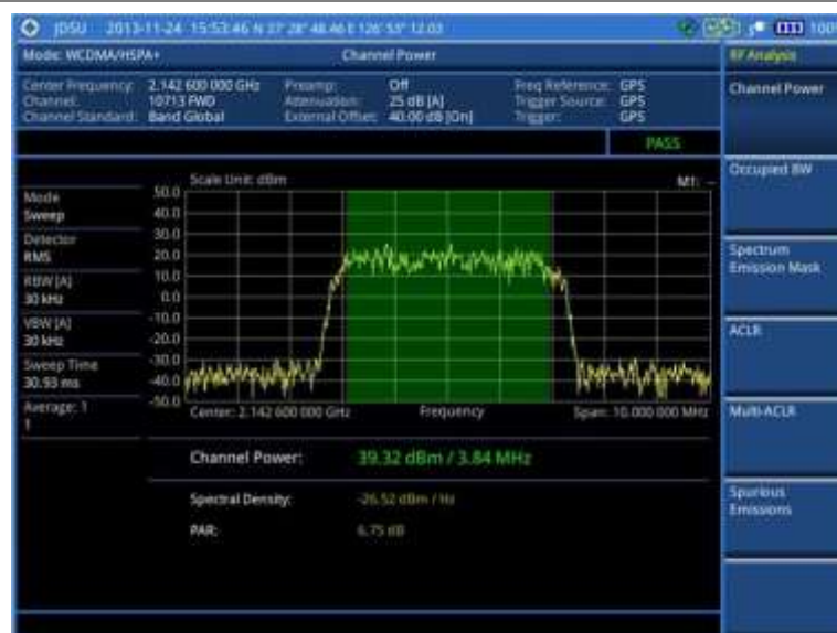
Figure 90 Channel power measurement with WCDMA/HSPA+ signal analyzer
