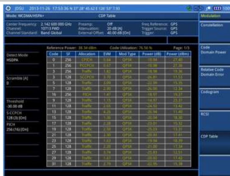
Figure 101 CDP Table measurement with WCDMA/HSPA+ signal analyzer
