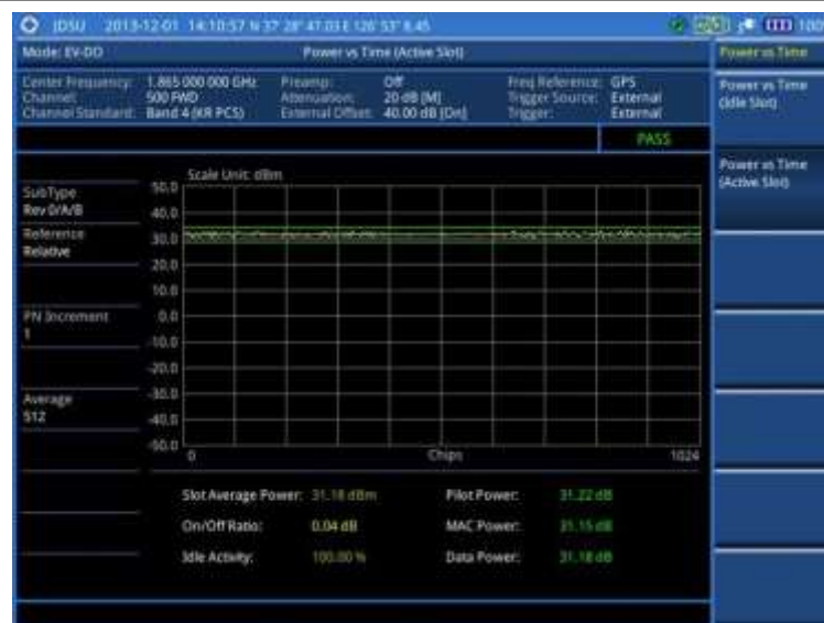
Figure 240 Power vs. time (active slot) measurement with EV-DO signal analyzer
