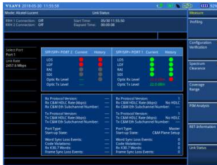
Figure 441 Example of verification of link status
