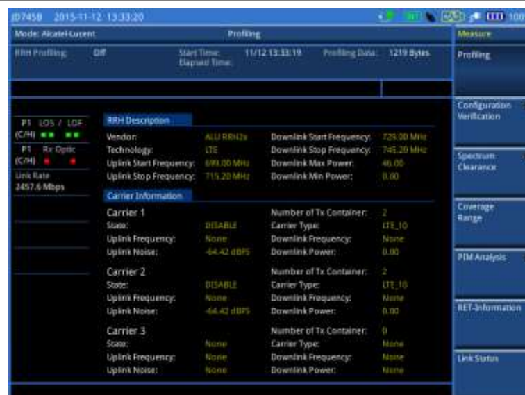
Figure 417 Example of RRH profiling results with carrier information
