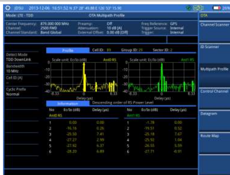
Figure 192 Multipath profile measurement with LTE-TDD OTA signal analyzer
