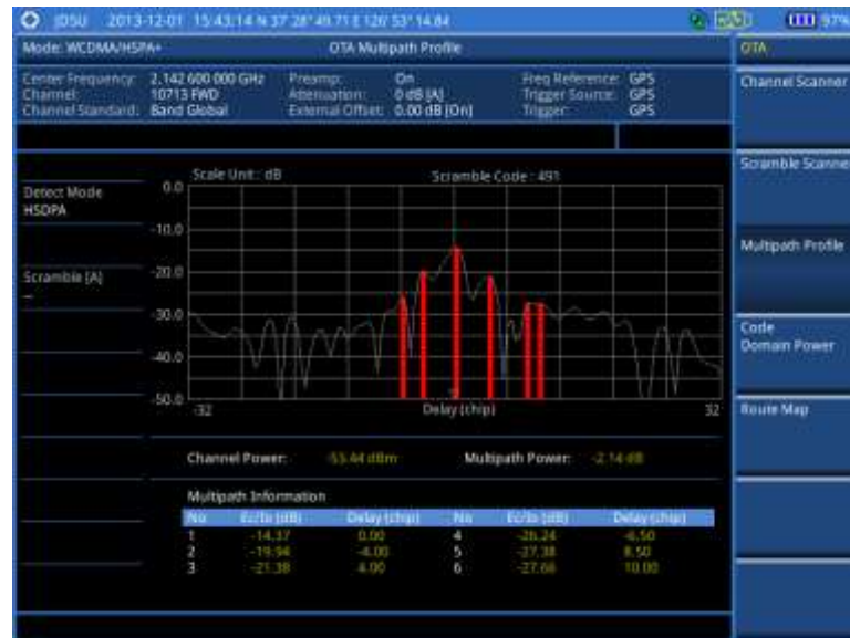
Figure 105 Multipath profile measurement with WCDMA/HSPA+ OTA signal analyzer
