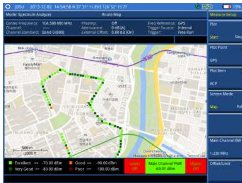
Figure 40 Route map measurement screen with GPS
