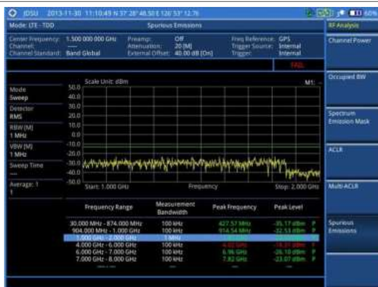
Figure 170 Spurious emissions measurement with LTE-TDD signal analyzer
