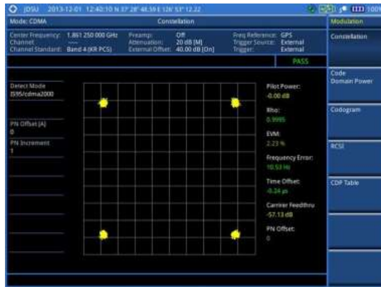
Figure 216 Constellation measurement with CDMA signal analyzer
