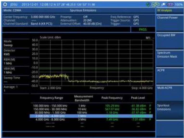
Figure 215 Spurious emissions measurement with CDMA signal analyzer
