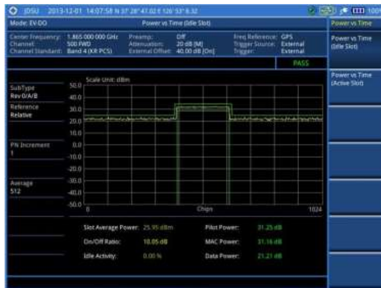
Figure 239 Power vs. time (idle slot) measurement with EV-DO signal analyzer
