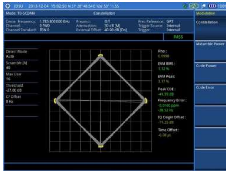
Figure 268 Constellation measurement with TD-SCDMA signal analyzer
