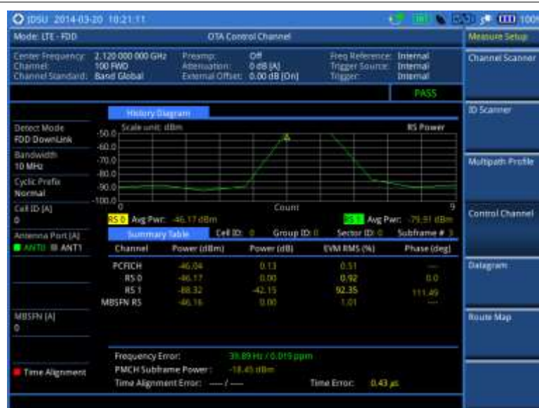
Figure 148 Control channel measurement with LTE-FDD OTA signal analyzer
