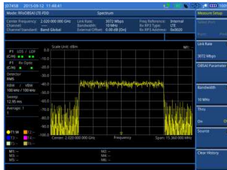
Figure 401 Spectrum measurement with RFoBSAI LTE-FDD signal analyzer
