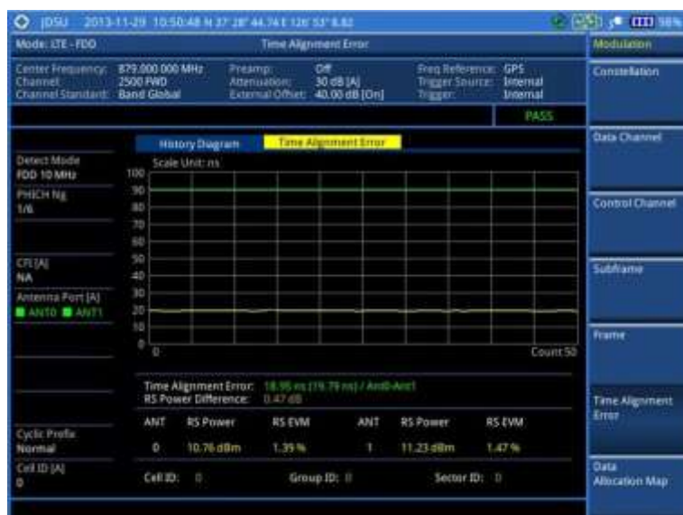
Figure 135 Time alignment error measurement with LTE-FDD signal analyzer
