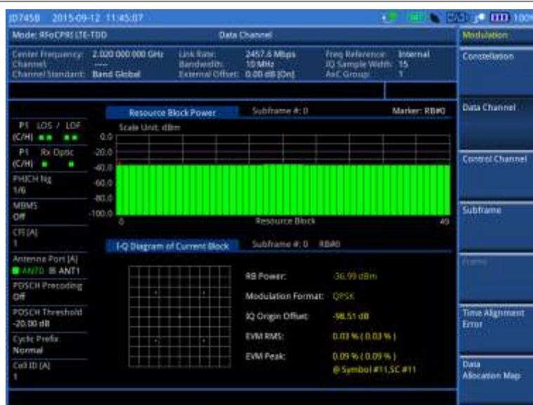
Figure 382 Data channel measurement with RFoCPRI LTE-FDD signal analyzer
