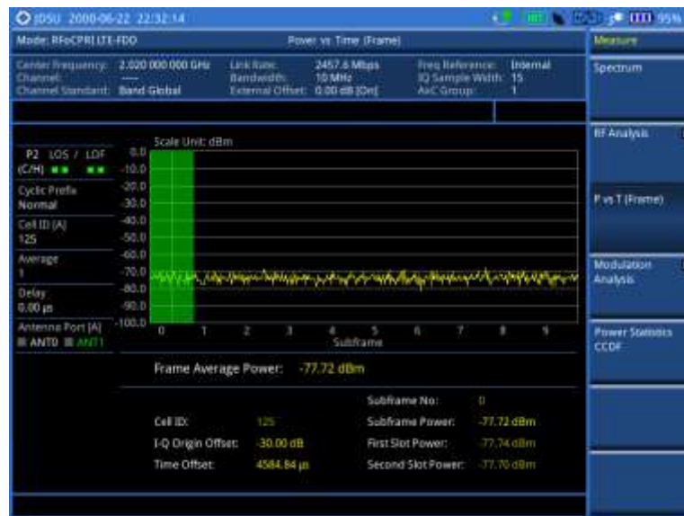
Figure 366 Power vs. time (frame) measurement with RFoCPRI LTE-FDD signal analyzer
