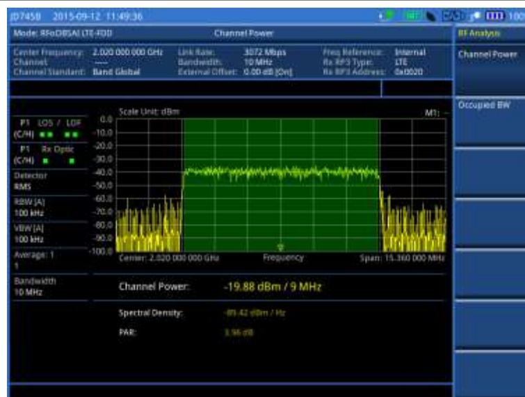
Figure 402 Channel power measurement with RFoBSAI LTE-FDD signal analyzer
