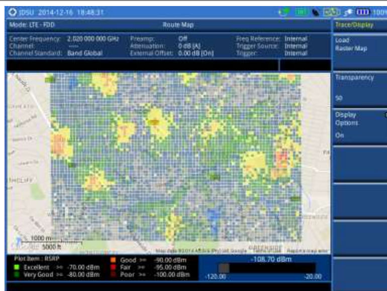
Figure 157 Raster image overlaid on the base map with LTE-FDD OTA signal analyzer
