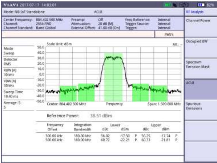
Figure 309 ACLR measurement with NB-IoT Standalone signal analyzer
