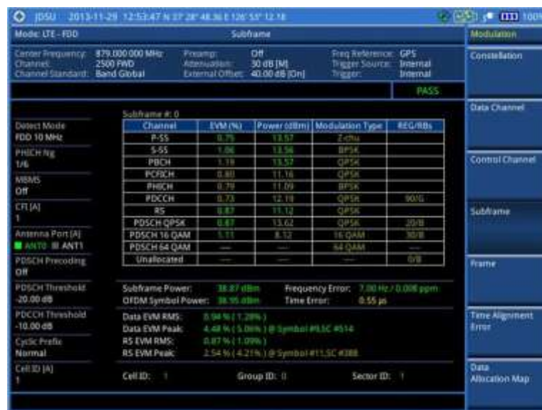
Figure 131 Subframe measurement with LTE-FDD signal analyzer (Chart On)
