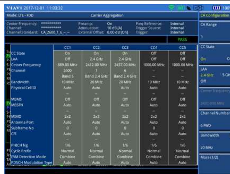
Figure 141 LAA (Licensed Assisted Access) measurement with LTE-FDD signal analyzer
