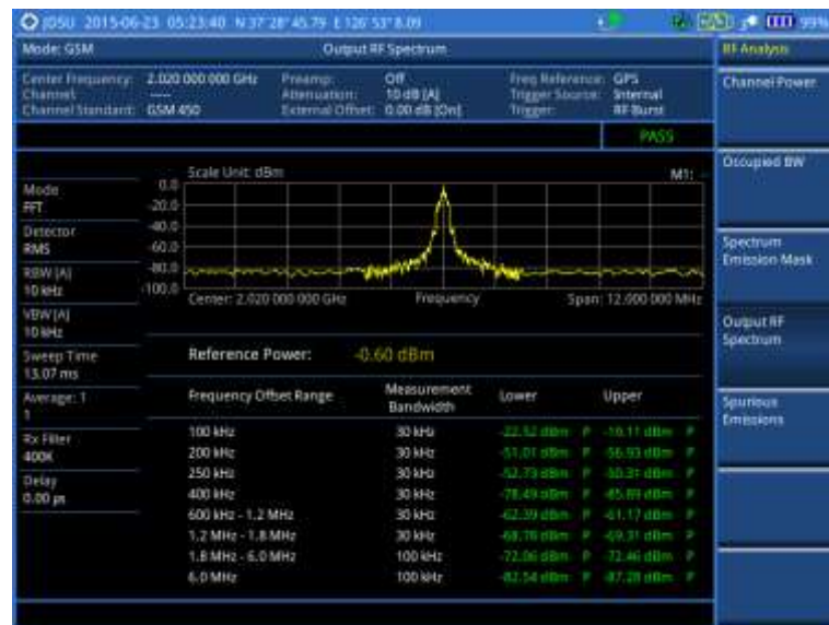
Figure 73 Output RF spectrum measurement with GSM signal analyzer
