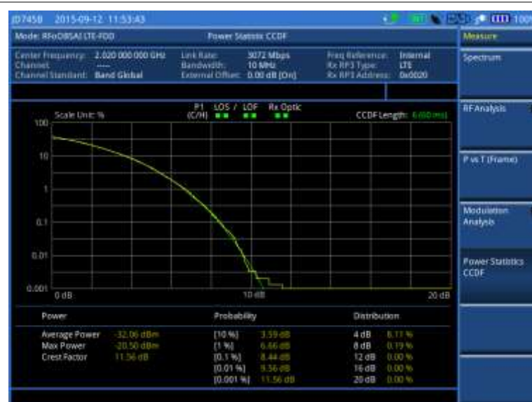
Figure 413 CCDF measurement with RFoBSAI LTE-FDD signal analyzer
