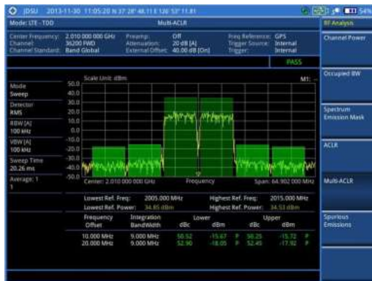
Figure 169 Multi-ACLR measurement with LTE-TDD signal analyzer
