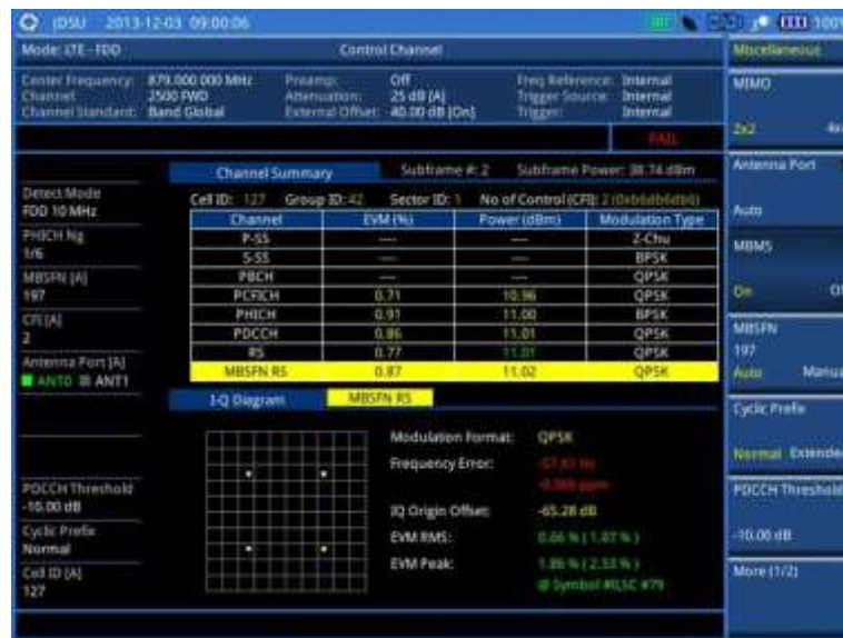
Figure 129 Control channel measurement with LTE-FDD signal analyzer (MBMS On)
