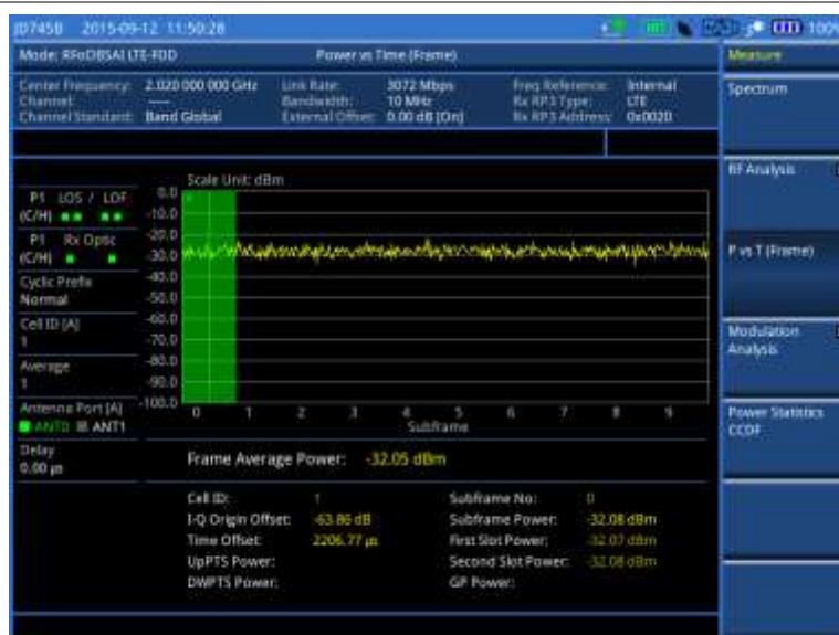
Figure 404 Power vs. time (frame) measurement with RFoBSAI LTE-FDD signal analyzer
