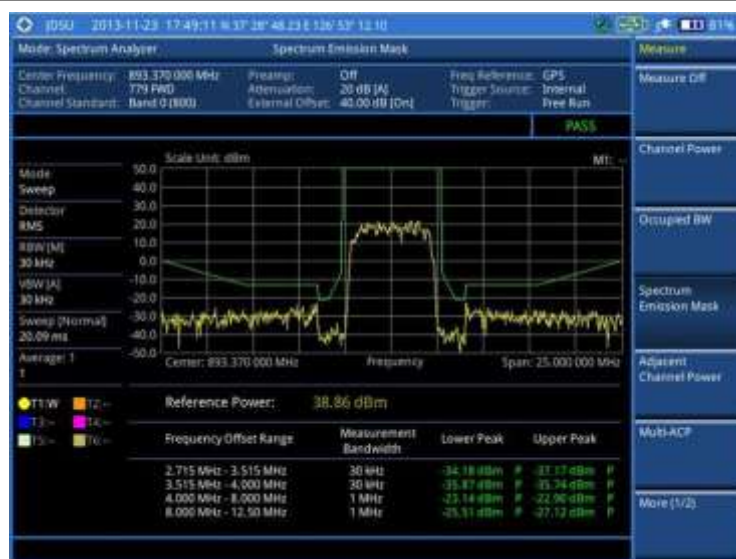
Figure 29 Spectrum emission mask measurement with spectrum analyzer (on 28 GHz downconverter)
