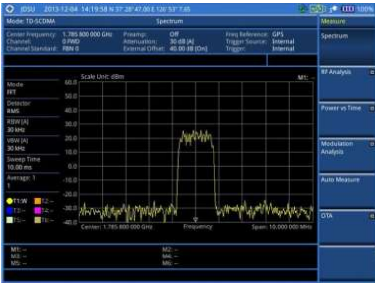
Figure 257 Spectrum measurement screen with TD-SCDMA signal analyzer
