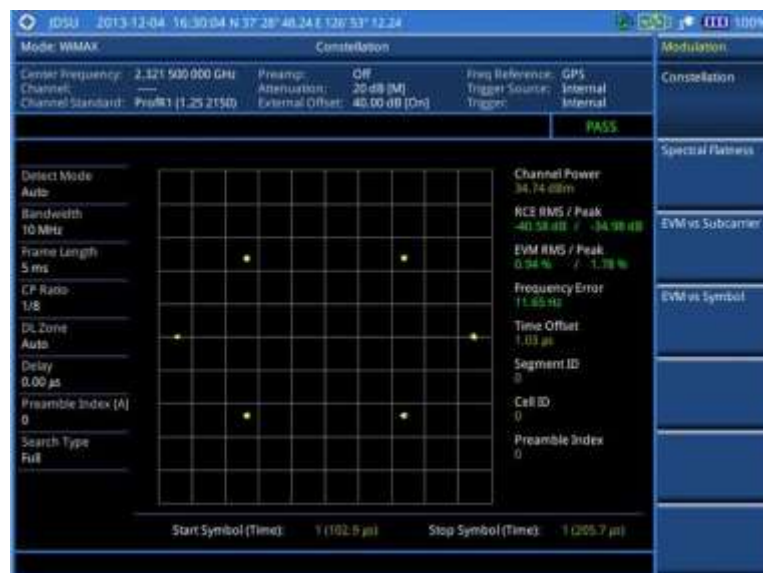
Figure 288 Constellation measurement with Mobile WiMAX signal analyzer
