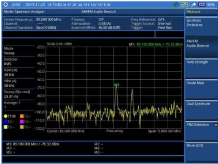
Figure 37 AM/FM audio demodulation with spectrum analyzer (on 28 GHz downconverter)
