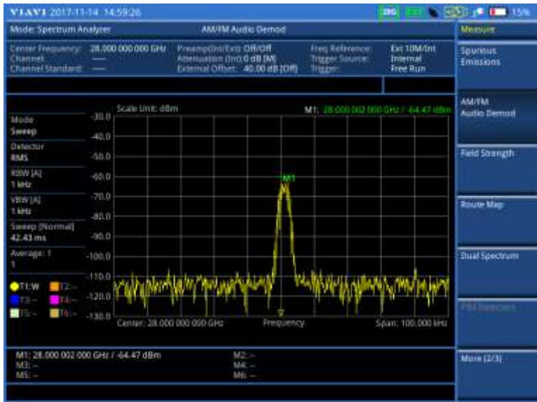
Figure 37 AM/FM audio demodulation with spectrum analyzer (on 28 GHz downconverter)
