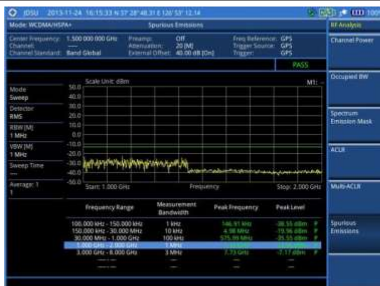
Figure 95 Spurious emissions measurement with WCDMA/HSPA+ signal analyzer
