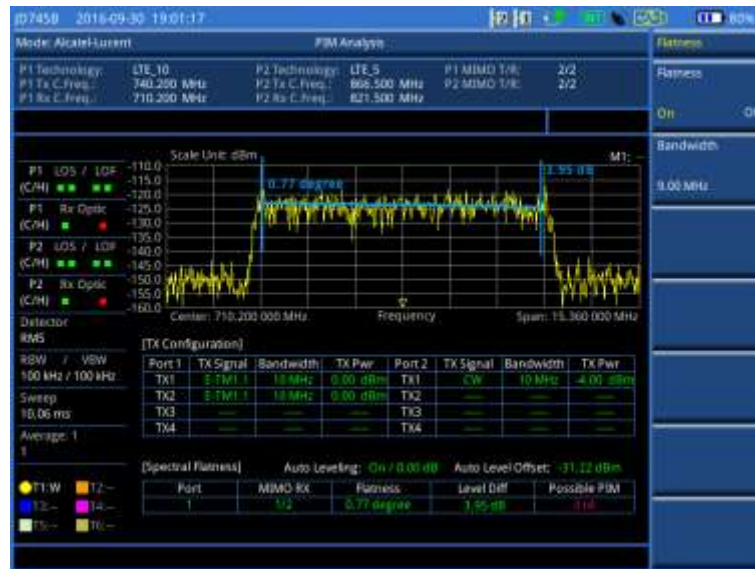
Figure 435 Example of Wideband Mode PIM analysis in Alcatel-Lucent BBU emulation
