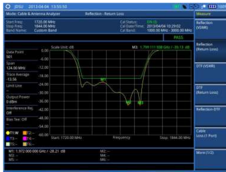
Figure 323 Reflection measurement in return loss scale
