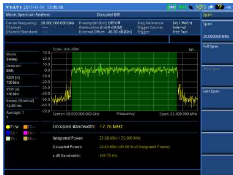
Figure 27 Occupied bandwidth measurement with spectrum analyzer (on 28 GHz downconverter)
