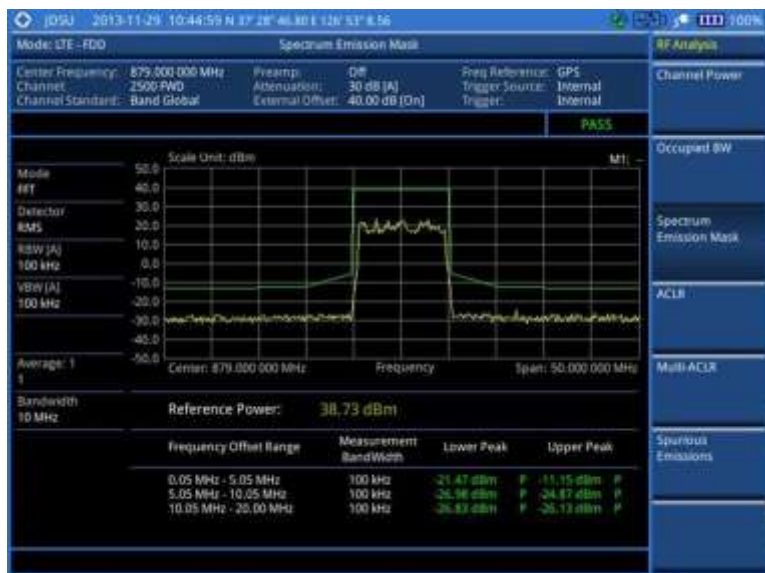
Figure 118 SEM measurement with LTE-FDD signal analyzer
