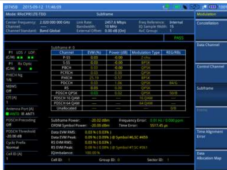
Figure 384 Subframe measurement (regular view) with RFoCPRI LTE-TDD signal analyzer
