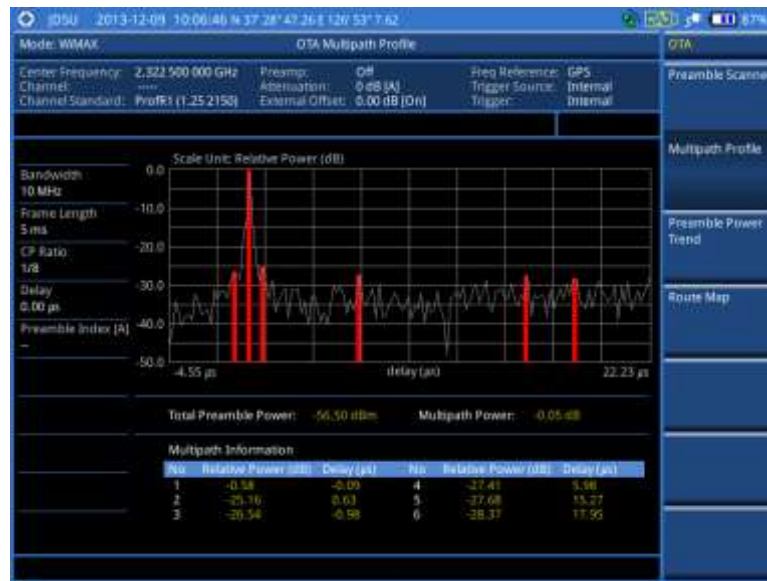
Figure 294 Multipath profile measurement with Mobile WiMAX OTA signal analyzer
