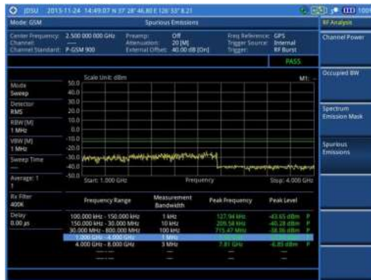
Figure 74 Spurious emissions measurement with GSM signal analyzer
