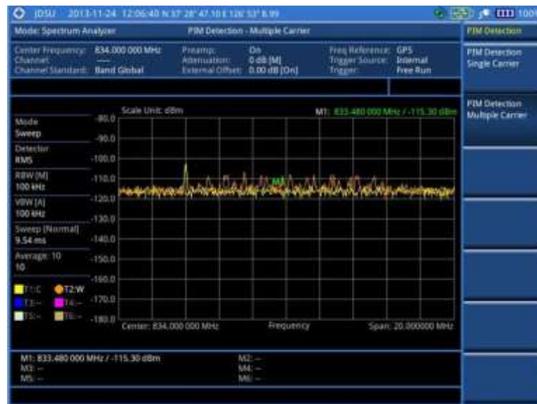
Figure 44 PIM detection for multiple carriers
