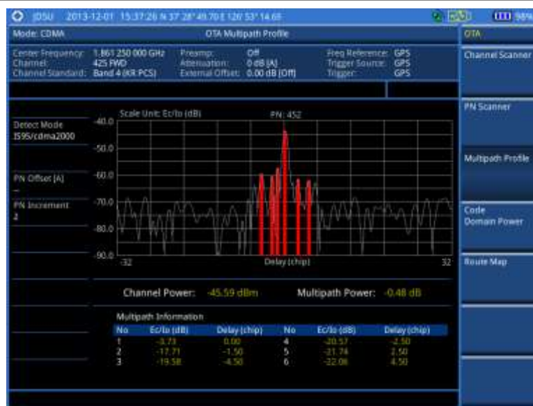
Figure 224 Multipath profile measurement with CDMA OTA signal analyzer
