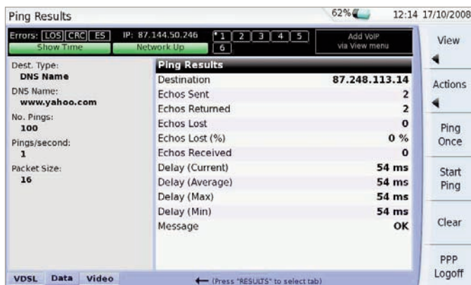
Figure 7: IP Ping test interface
