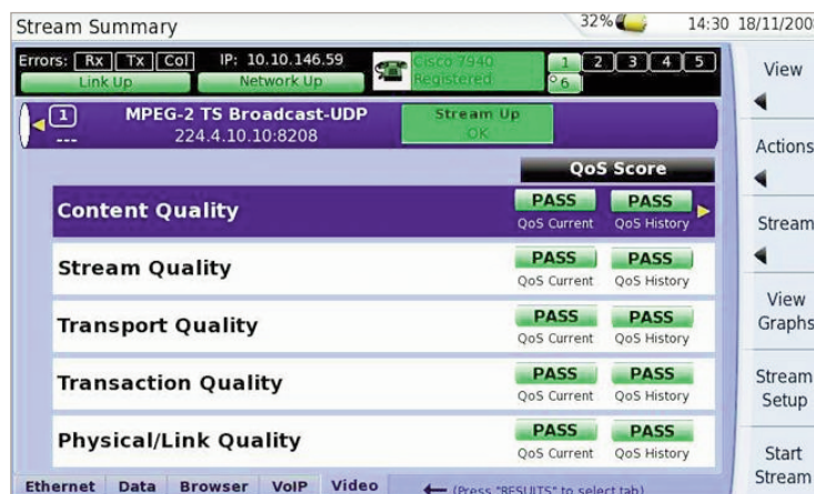
Figure 5: Example of IPTV Summary test screen
