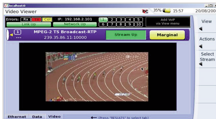
Figure 4: Example of IPTV Video Stream test
