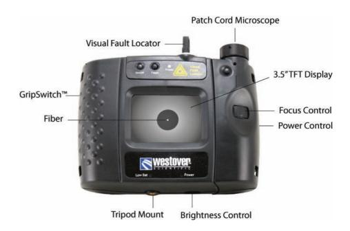
The FMV Series Video Viewer combines performance, versatility and value. Used for visual field inspection of optical fiber, the FMV Video Viewer incorporates a variety of features that enable efficient patch cord inspection.
