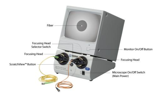
The FVDW Series microscopes utilize coaxial illumination to provide the user with a critical view of fine scratches, making them the ideal choice for factory post-polish inspection, component assembly, and QC environments. The FVDW systems feature an attached 9" monitor that is inclined backward 22.5° and accept all FMA-Series adapters. Each microscope has two heads, ideal for inspecting:
