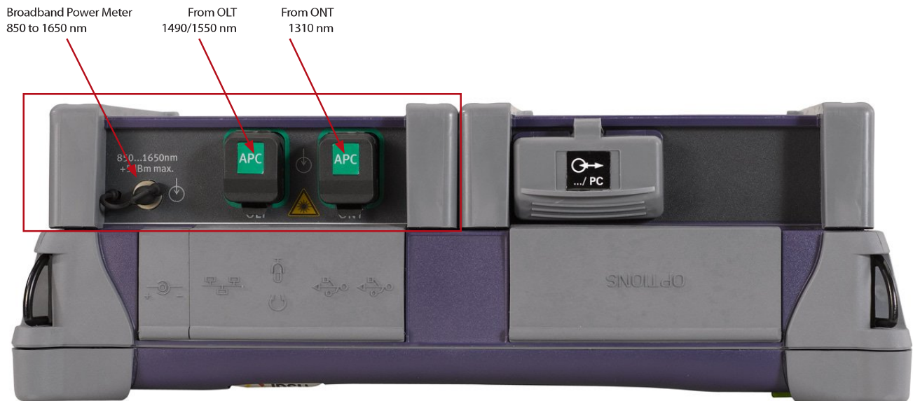
T-BERD/MTS-4000 with OLP-4057 module
