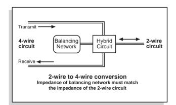
For the hybrid to work correctly the impedance of the balancing network should match that of the 2-wire circuit. In practice the 2-wire impedance depends on the loop length and conditions so it is difficult to balance correctly. This results in echoes and return losses on both sides.
