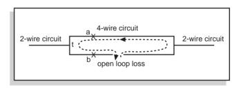
"Semi-Loop Loss: The transmission loss between points 'a' and 'b' of the 4-wire termination independent of whether there exists or not a physical point 't'." CCITT Blue Book Vol. III G.100 4.11
