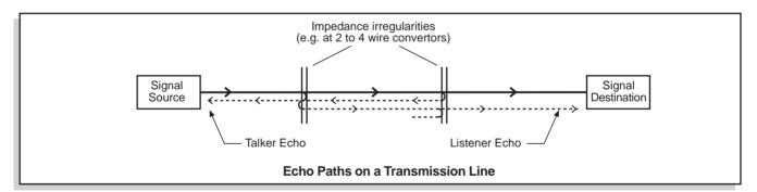
Impedance mismatches in communications circuits cause problems because signals are reflected back to the source from each mismatch. This can result in a loss of power transfer and interference with, or corruption of, the signal.
