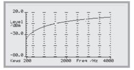
When the measurement <RUN> softkey is pressed the Level vs Frequency graph will be displayed showing the return loss against frequency. Stopping the test enables the cursor to be used to read off return loss at a particular frequency.
