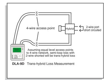
The trans-hybrid loss is determined by shorting the 2-wire port of the hybrid and measuring the circuit loss on the 4-wire side. In the ideal case this would be -6dBm.
