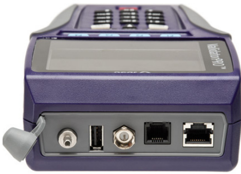
Test fiber and copper (telco, network &amp; coax) cables
