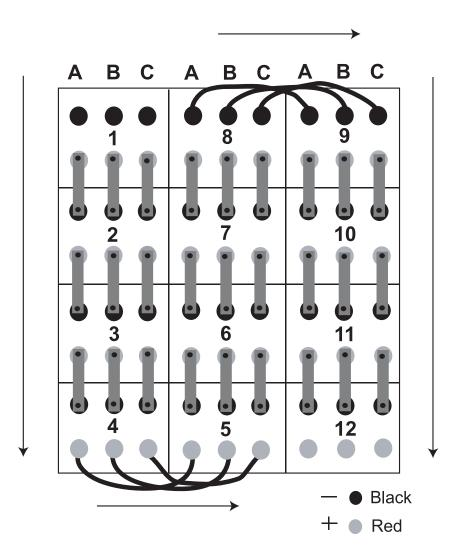
Figure 4: Pattern for testing jars in a string
