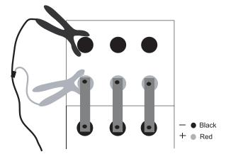
Figure 5: Attaching the cable to jar posts
