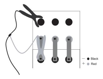
Figure 6. Attaching the cable to a strap
