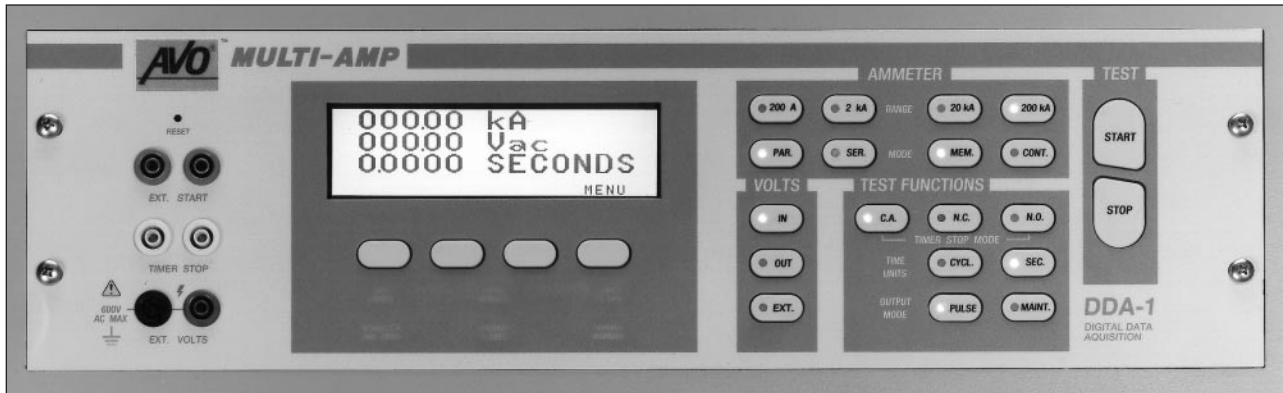
Model DDA-1600 uses the Model DDA-1 Digital Data Acquisition Instrumentation and Control System. This system offers the latest in digital signal processing technology to control the test set and measure reactions of the breaker under test.
