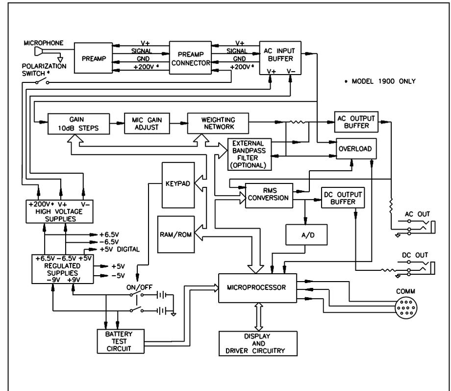
Figure 16. Block Diagram of the Model 1900
