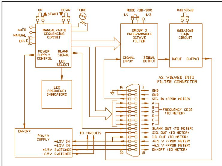
Figure 33. Block Diagram of Models OB-100 and OB-300
