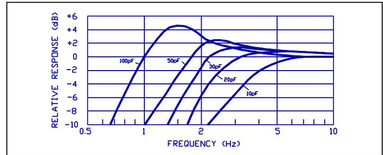
Figure 20. Effect of Microphone Output Capacitance on Preamp Low Frequency Response
