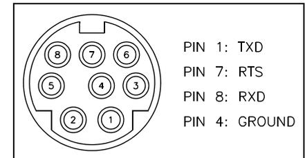
Figure 12. COMM Jack Pinout for RS-232 Communication
