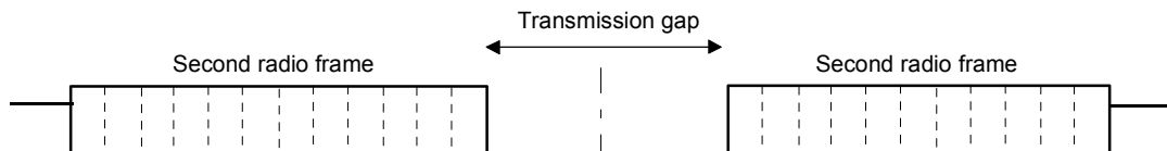
Fig. 4-36 Envelope of compressed mode signal with double-frame method
