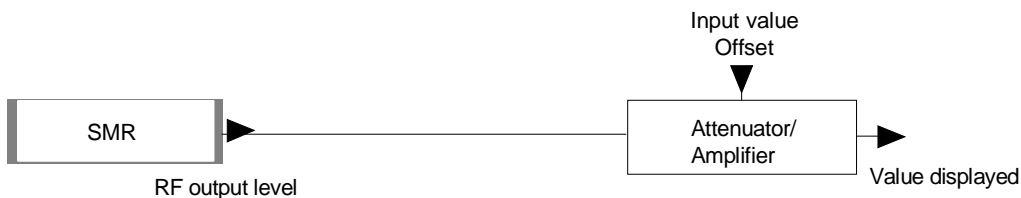
Fig. 4-4 Typical setup with level offset
