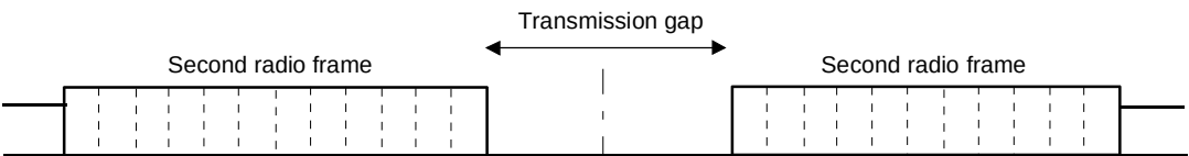
Fig. 4-37 Envelope of compressed mode signal with double-frame method
