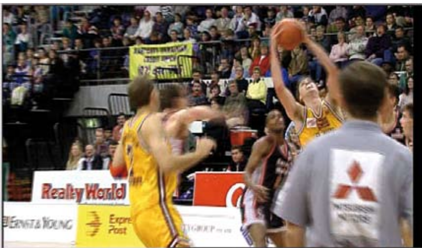
Clearly visible blocking effects on digitally coded TV picture and – by comparison – picture without blocking
