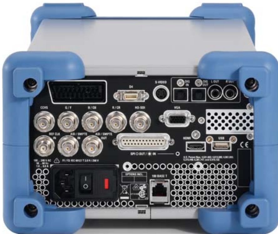
Rear view of the R&S®DVSG showing interfaces
